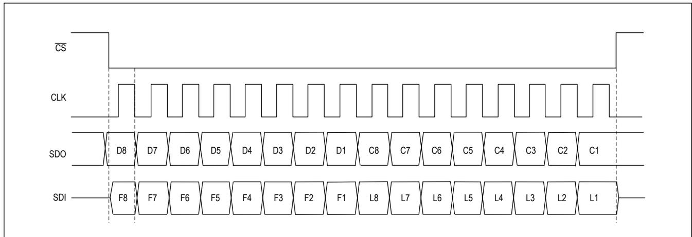
Figure 9. SPI Cycle in 16-Bit Direct SPI Mode
