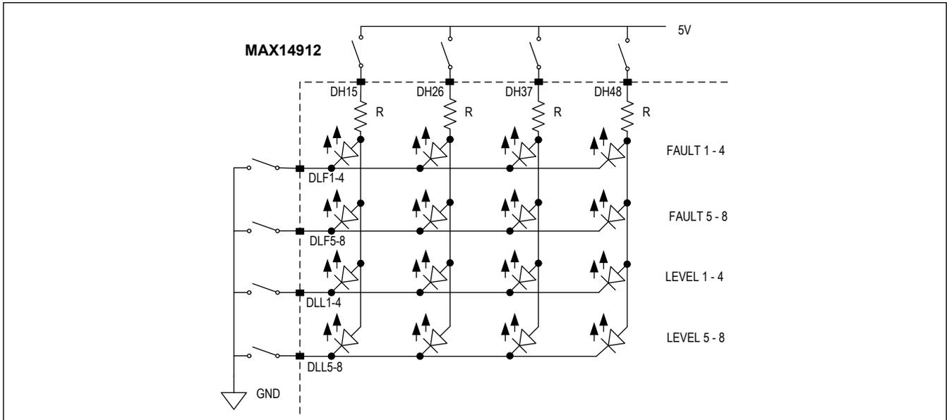
Figure 6. LED Output Status and Fault-Detection Matrix
