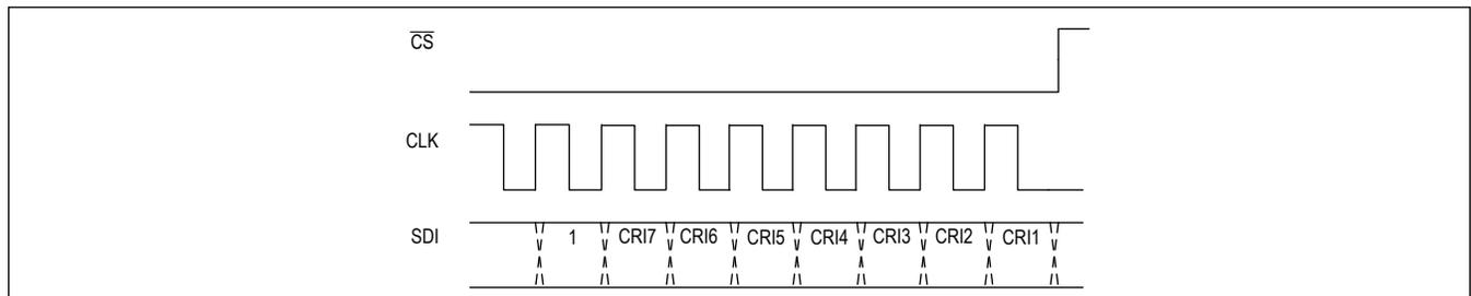
Figure 10. SDI Check Byte Expected from Controller
