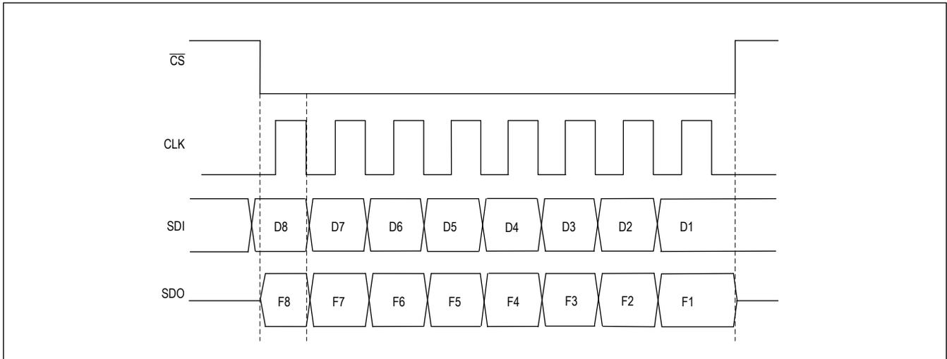
Figure 8. SPI Cycle in 8-Bit Direct SPI Mode
