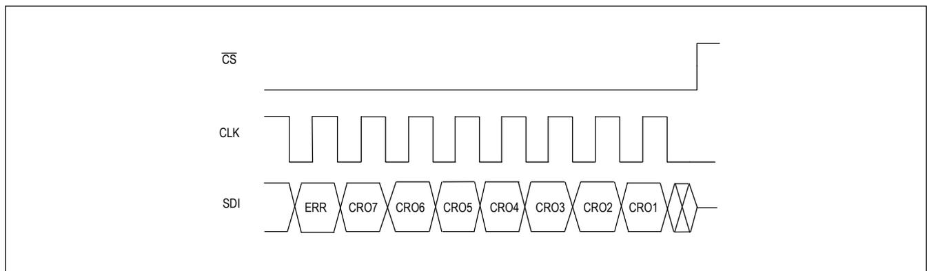
Figure 11. SDO Check Byte Sent by Device
