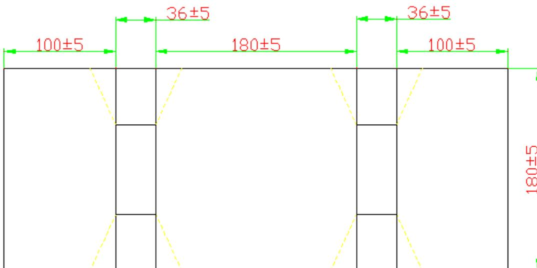
e. Drawing of middle size carton in developed view
