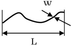
The diagram shows a wavy line representing a linear scratch. A horizontal double-headed arrow below the line is labeled 'L', representing the length of the scratch. A vertical double-headed arrow pointing to the peak of the wavy line is labeled 'W', representing the width of the scratch.
