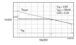
Figure 2. Backup Time Supporting 50mA Load
