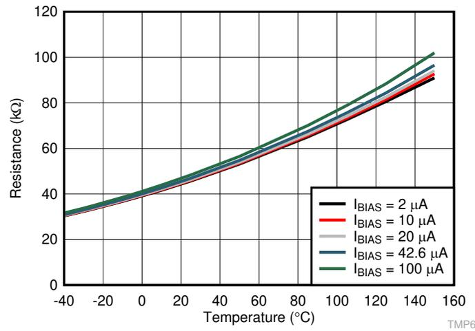
Figure 9-8. TMP64 Temperature Voltage With Varying Current Sources
