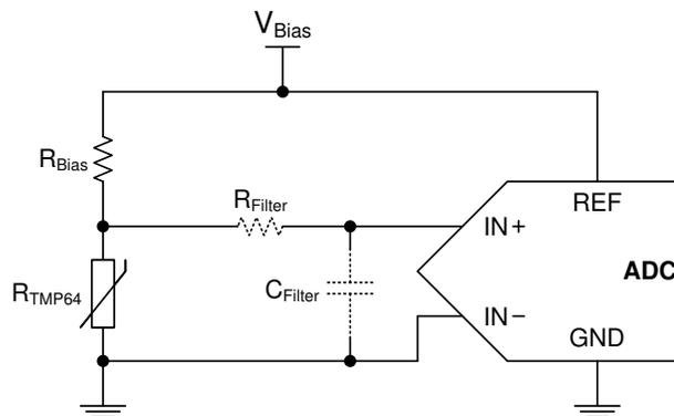
**Figure 9-2. TMP64 Voltage Divider With an ADC**
