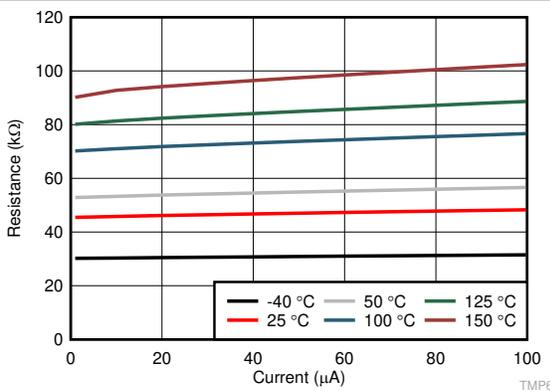
**Figure 7-5. Supply Dependence Resistance vs. Bias Current**
