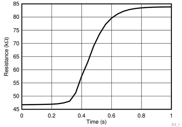
TMP64: Stirred Liquid. Temperature: 25 °C to 125 °C
