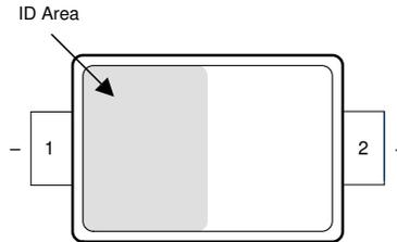
**Figure 6-2. DYA Package 2-Pin SOT-5X3 Top View**
