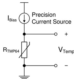
**Figure 9-3. TMP64 Biasing Circuit With Current Source**
