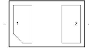
**Figure 6-1. DEC Package 2-Pin X1SON Bottom View**
