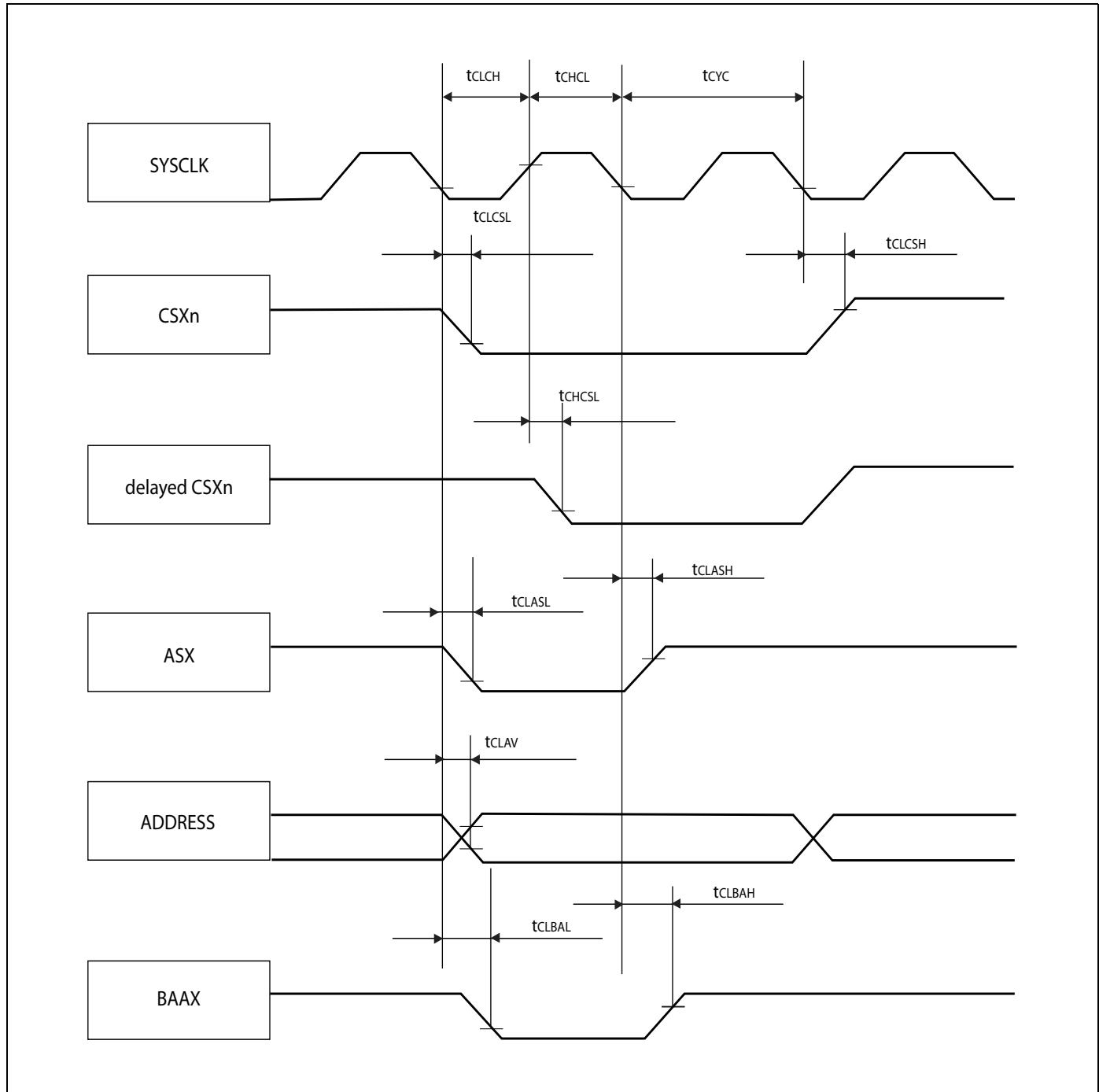
*Synchronous/Asynchronous read access*
