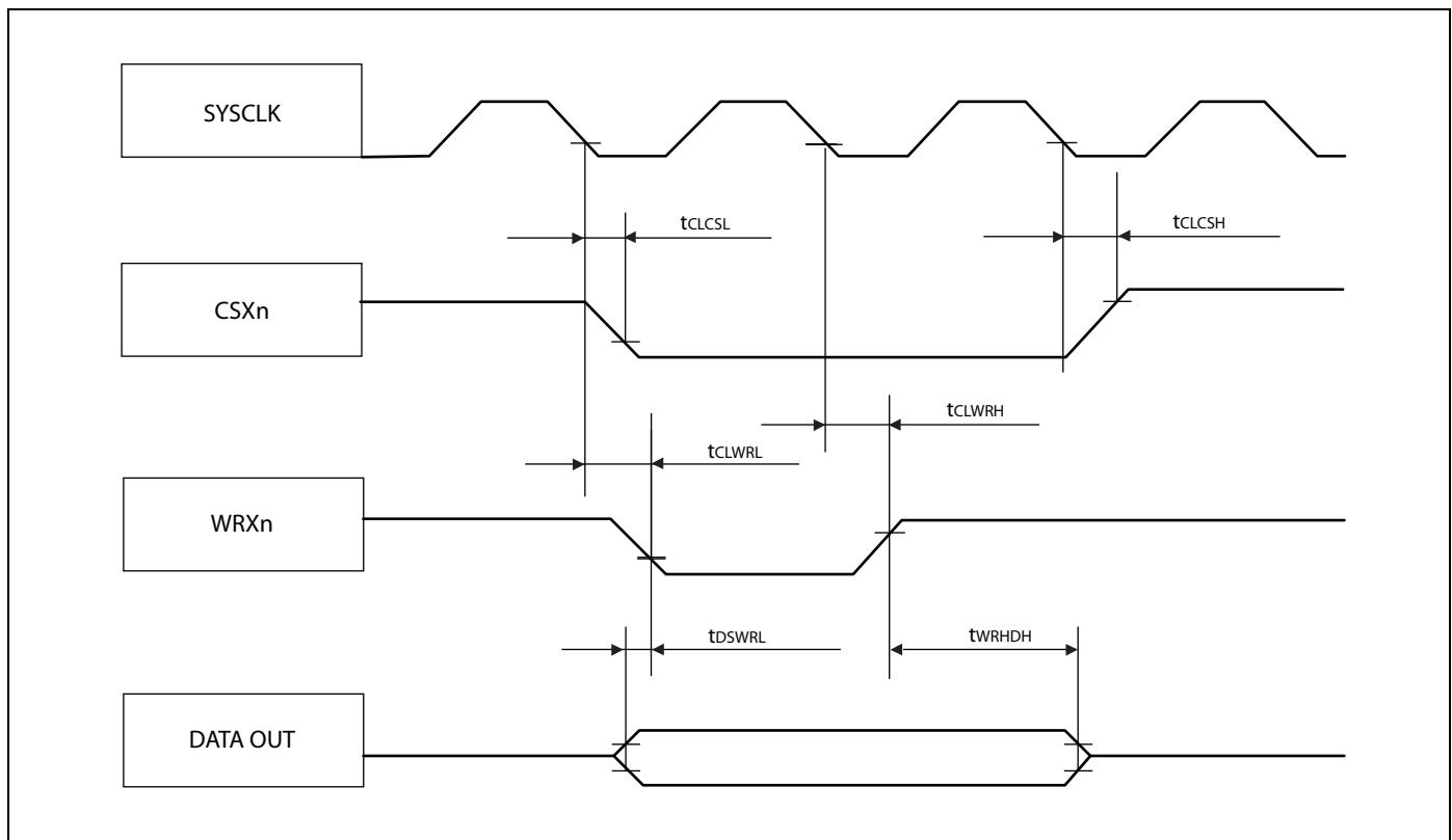
*Asynchronous write access*
