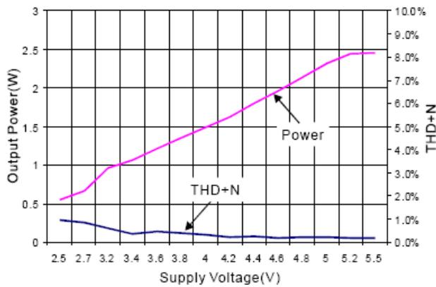
**Typical Performance Characteristics** (cont.) (@ $T_A = +25^\circ\text{C}$ ,  $V_{DD} = 5\text{V}$ ,  $G_V = 20\text{dB}$ ,  $R_L = 8\Omega$ , unless otherwise specified.)
