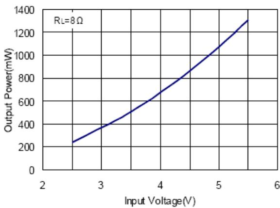
12. Output Power VS Supply Voltage
