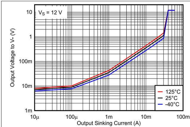
**Figure 7-7. Output Voltage vs. Output Sinking Current, 12 V**
