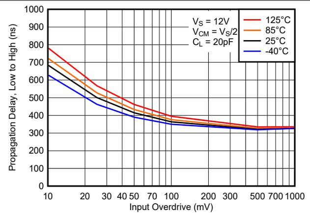
Figure 7-16. Propagation Delay, Low to High, 12V
