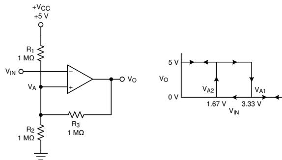
Figure 9-3. TLV181xin an Inverting Configuration With Hysteresis
