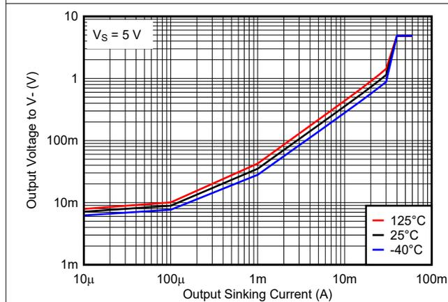
**Figure 7-5. Output Voltage vs. Output Sinking Current, 5 V**
