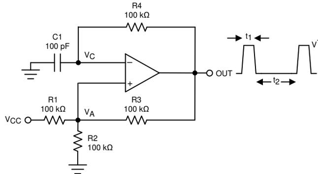
**Figure 9-9. Square-Wave Oscillator**
