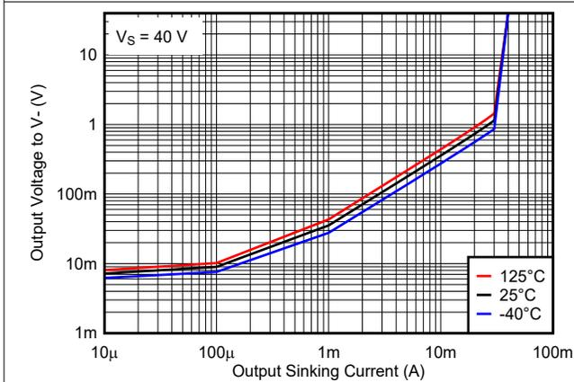
**Figure 7-9. Output Voltage vs. Output Sinking Current, 40 V**
