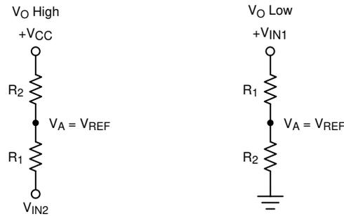
**Figure 9-6. Non-Inverting Configuration Resistor Networks**
