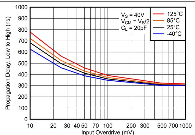
Figure 7-18. Propagation Delay, Low to High, 40V
