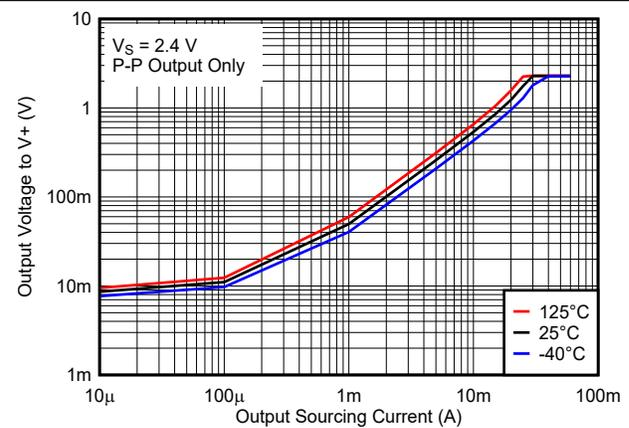
**Figure 7-4. Output Voltage vs. Output Sourcing Current, 2.4 V**
