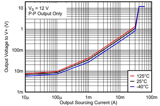
**Figure 7-8. Output Voltage vs. Output Sourcing Current, 12 V**
