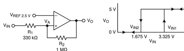
**Figure 9-5. TLV181x in a Non-Inverting Configuration With Hysteresis**
