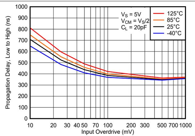
Figure 7-14. Propagation Delay, Low to High, 5V
