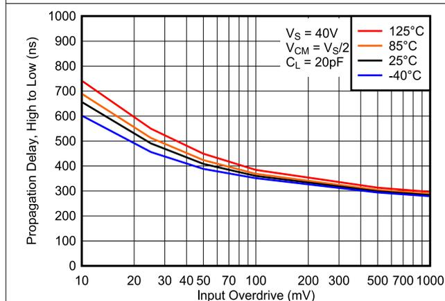
Figure 7-17. Propagation Delay, High to Low, 40V
