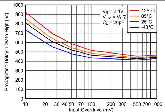
**Figure 7-12. Propagation Delay, Low to High, 2.4V**
