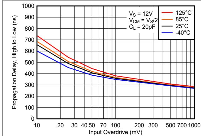
Figure 7-15. Propagation Delay, High to Low, 12V
