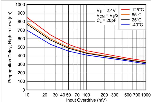
**Figure 7-11. Propagation Delay, High to Low, 2.4V**
