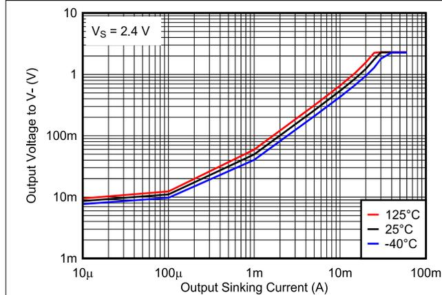
**Figure 7-3. Output Voltage vs. Output Sinking Current, 2.4 V**
