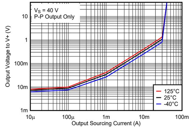
**Figure 7-10. Output Voltage vs. Output Sourcing Current, 40 V**
