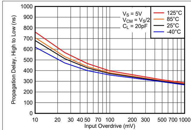
Figure 7-13. Propagation Delay, High to Low, 5V
