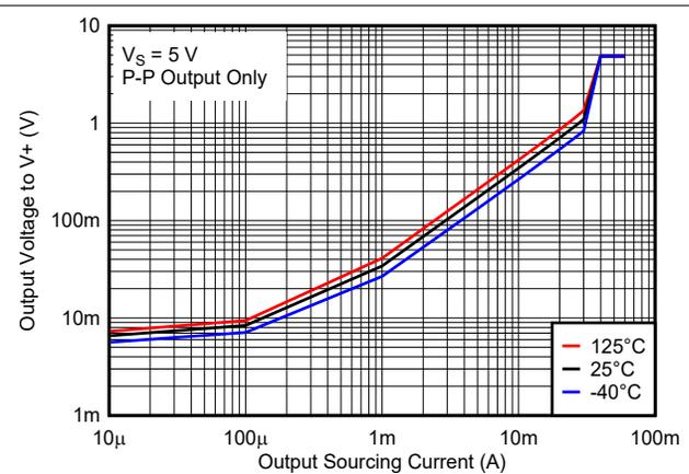
**Figure 7-6. Output Voltage vs. Output Sourcing Current, 5 V**
