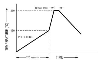
Wave soldering is suitable for 1210 size models.
