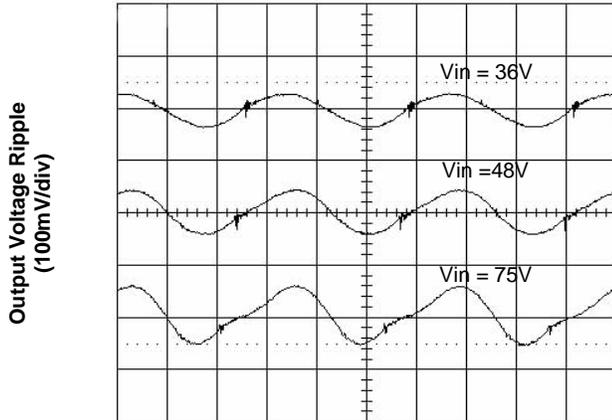
Figure 3. Output Ripple Voltage at Full Load
