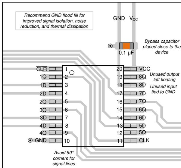
Figure 11-1. Example Layout for the SN74HCS273 PW Package
