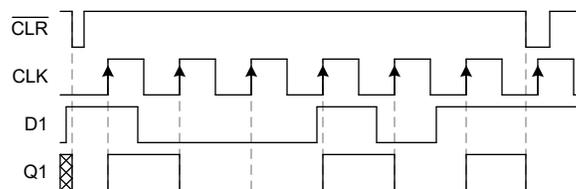
**Figure 9-2. Application Timing Diagram, One Data Channel Shown**
