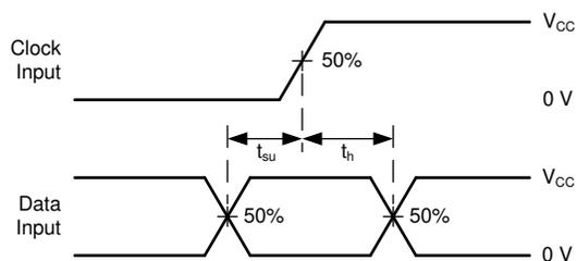
**Figure 7-3. Voltage Waveforms, Setup and Hold Times**
