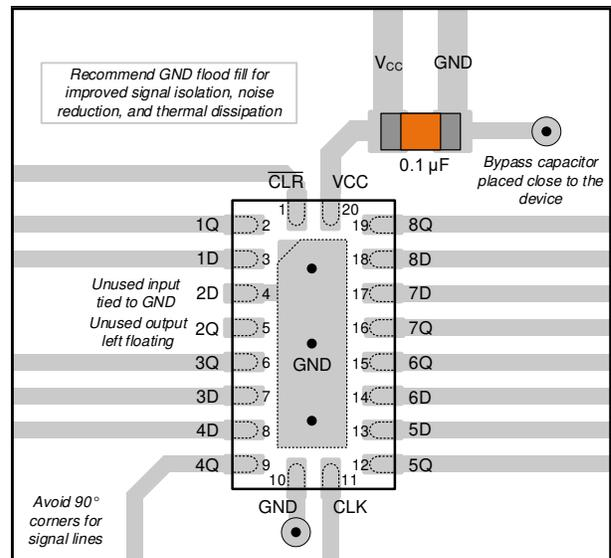
Figure 11-2. Example Layout for the SN74HCS273 RKS Package
