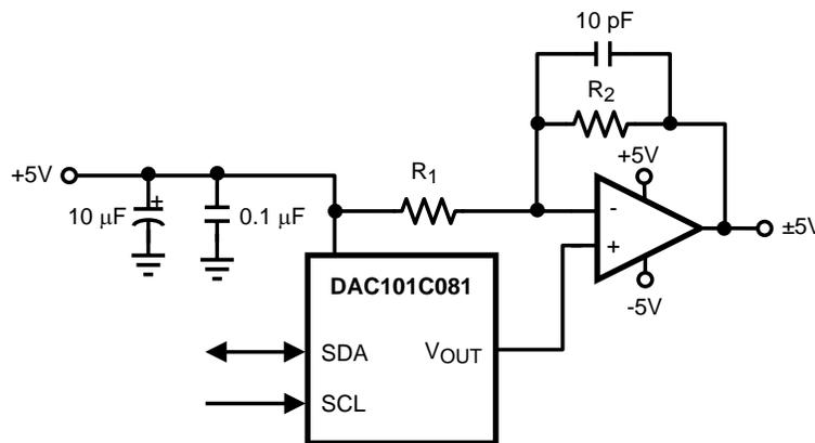
**Figure 27. Bipolar Operation**
