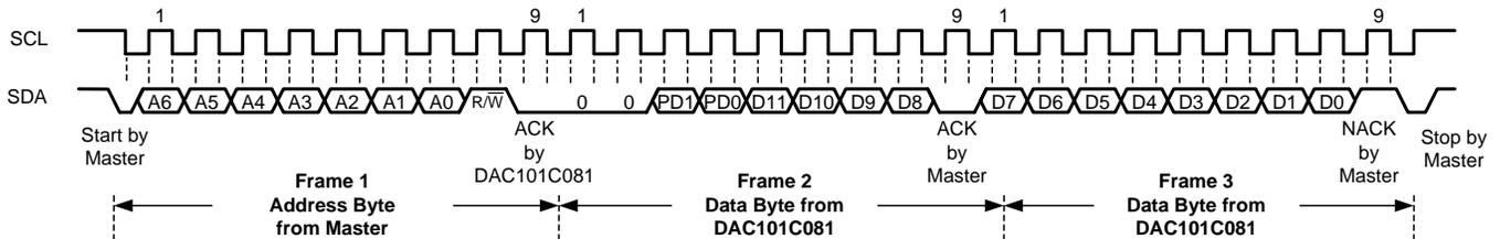
Figure 25. Typical Read from the DAC Register
