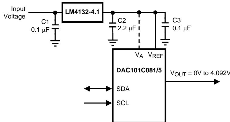
Figure 31. The LM4132 as a Power Supply
