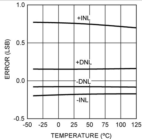
Figure 6. INL/DNL vs Temperature at  $V_A = 5$  V
