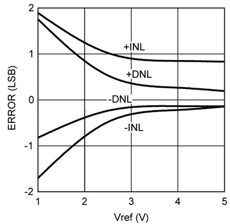
Figure 8. INL/DNL vs  $V_{REFIN}$  at  $V_A = 5$  V
