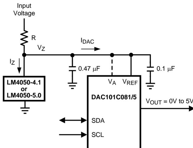
**Figure 32. The LM4050 as a Power Supply**
