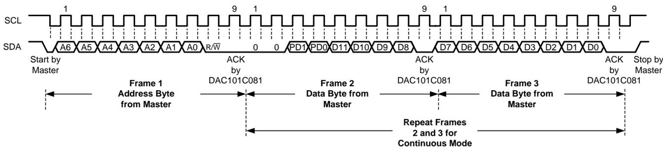
Figure 24. Typical Write to the DAC Register
