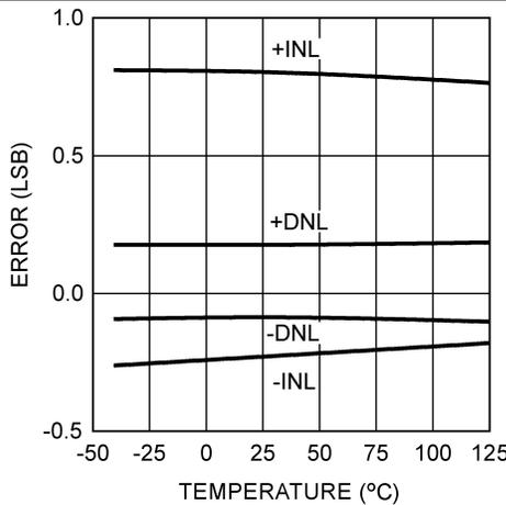
Figure 5. INL/DNL vs Temperature at  $V_A = 3.0$  V
