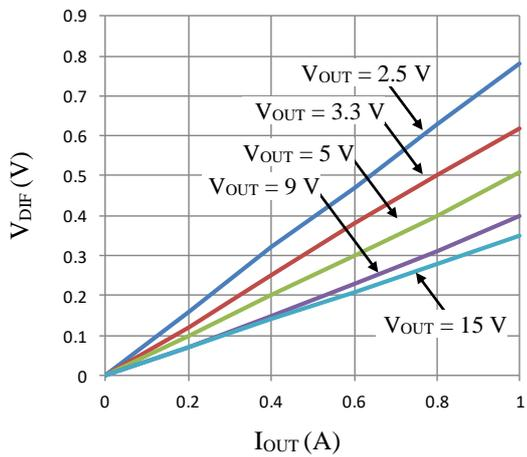
Figure 6-3. Dropout Voltage, V<sub>DIF</sub> vs. Output Current, I<sub>OUT</sub>
