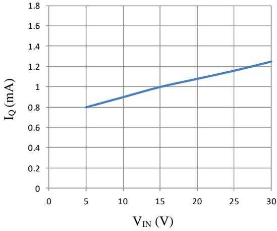
Figure 6-1. Quiescent Current, I<sub>Q</sub> vs. Input Voltage, V<sub>IN</sub>
