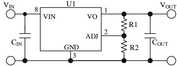
Figure 13-1. ADJ Pin Peripheral Circuit
