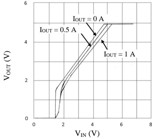
Figure 6-2. Output Voltage, V<sub>OUT</sub> vs. Input Voltage, V<sub>IN</sub>
