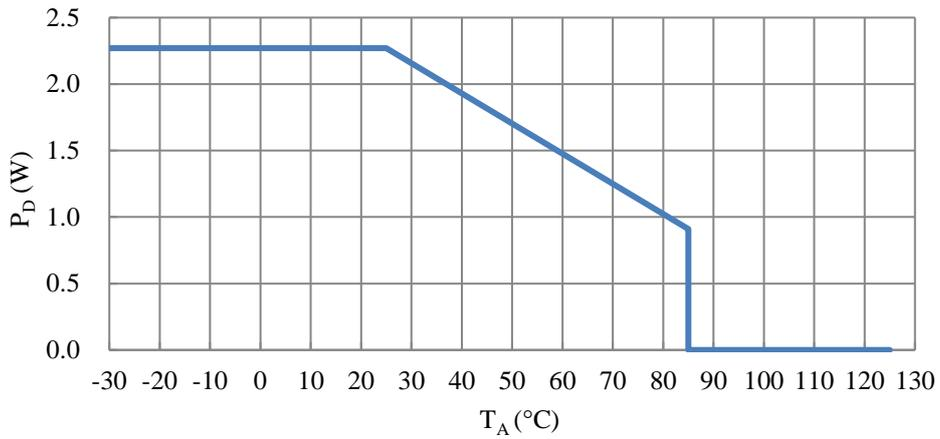
Figure 7-1. Allowable Power Dissipation, P<sub>D</sub> vs. Ambient Temperature, T<sub>A</sub>
