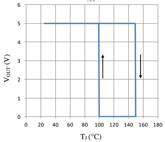
Figure 6-8. Thermal Shutdown Characteristics
