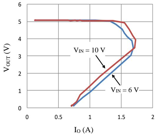
Figure 6-6. Overcurrent Protection Characteristics
