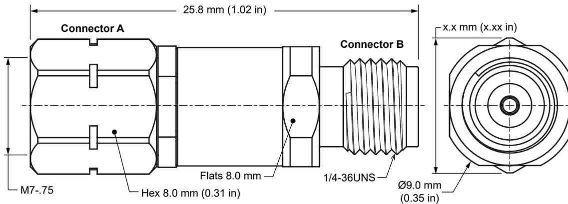
Figure 1. Product Dimensions for the ADP-2.4M-2.92F Adapter
