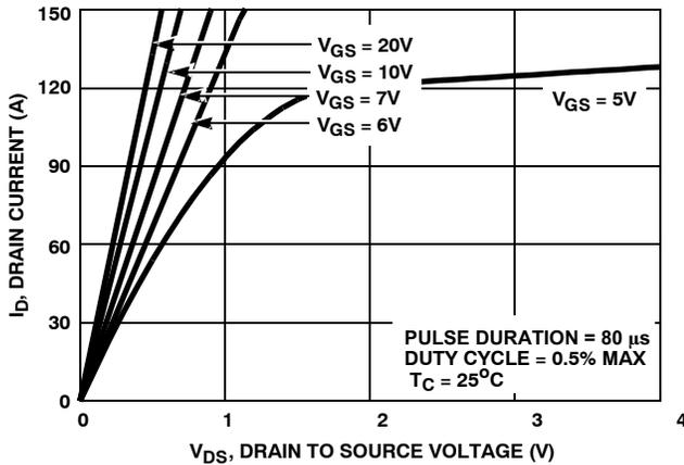
Figure 7. Saturation Characteristics
