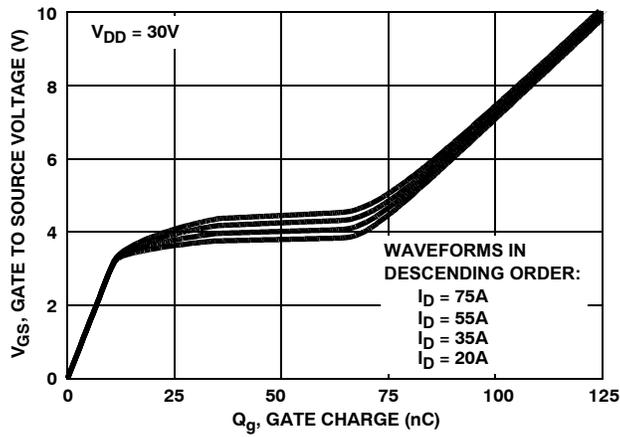
Figure 13. Gate Charge Waveforms for Constant Gate Currents
