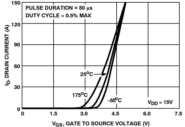
Figure 8. Transfer Characteristics
