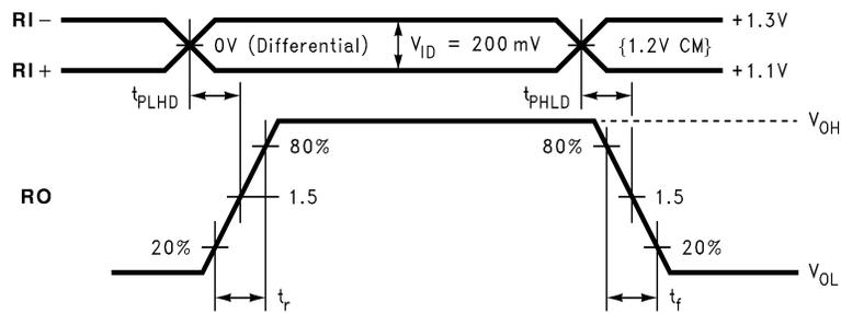
Figure 8. Receiver Propagation Delay and Transition Time Waveforms
