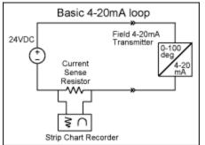
Figure 1. Basic architecture of a 4-20mA current loop.
