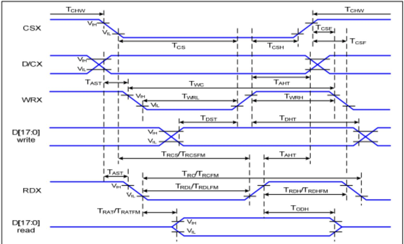
Figure 6.2: Parallel Interface Timing Characteristics (8080-Series MCU Interface)
