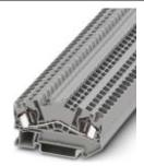
Feed-through terminal block, Connection method: Spring-cage connection, Cross section: 0.08 mm² - 6 mm², AWG: 28 - 10, Width: 6.2 mm, Color: blue, Mounting type: NS 35/7,5, NS 35/15
