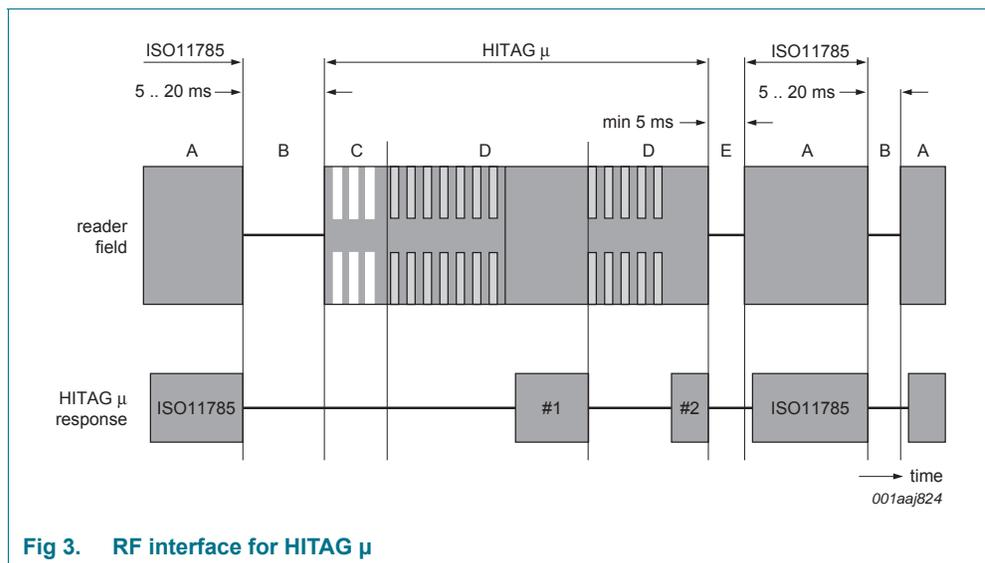
Fig 3. RF interface for HITAG  $\mu$
