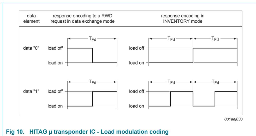
**Fig 10. HITAG  $\mu$  transponder IC - Load modulation coding**
