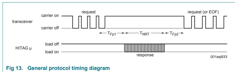
**Fig 13. General protocol timing diagram**
