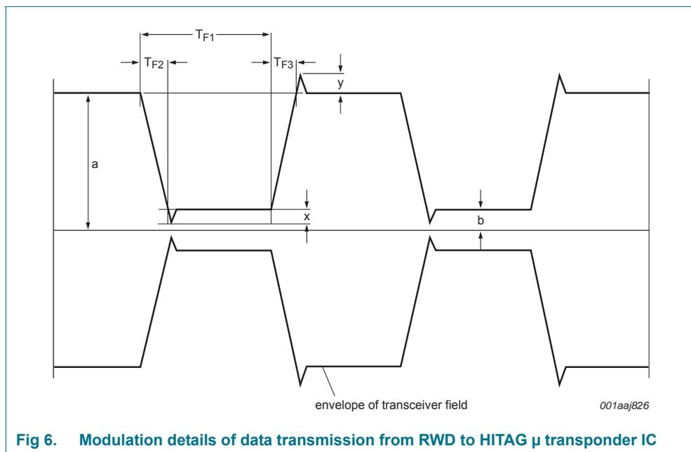
Fig 6. Modulation details of data transmission from RWD to HITAG  $\mu$  transponder IC
