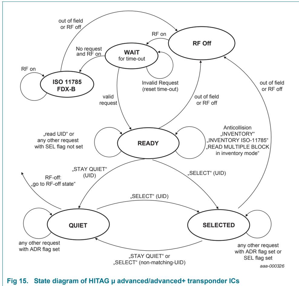
Fig 15. State diagram of HITAG  $\mu$  advanced/advanced+ transponder ICs
