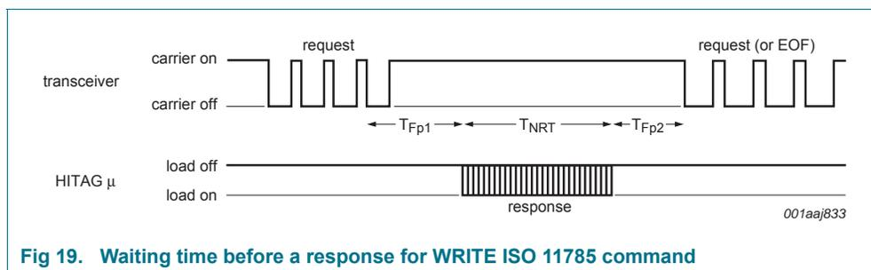
**Fig 19. Waiting time before a response for WRITE ISO 11785 command**
