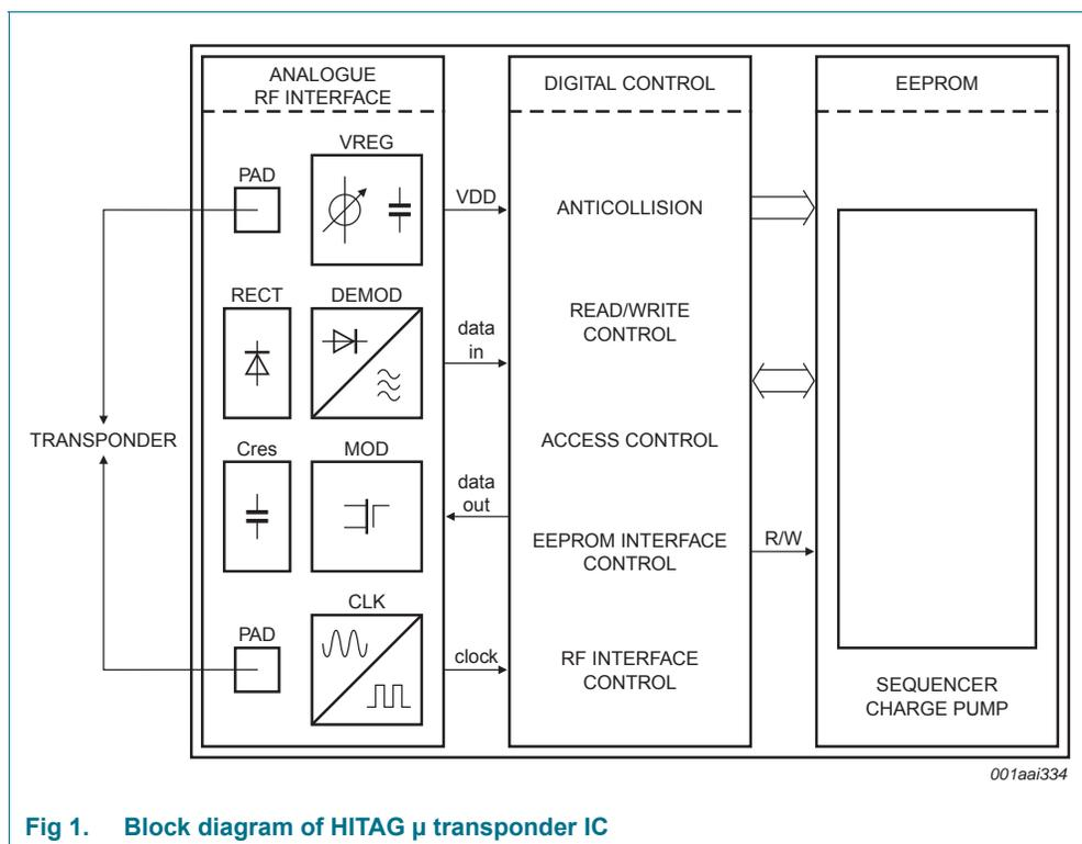
**Fig 1. Block diagram of HITAG  $\mu$  transponder IC**
