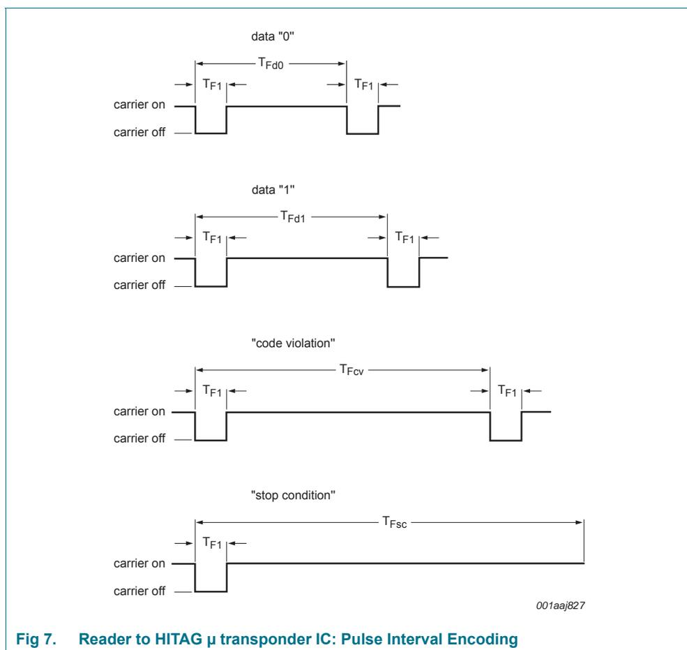
**Fig 7. Reader to HITAG  $\mu$  transponder IC: Pulse Interval Encoding**
