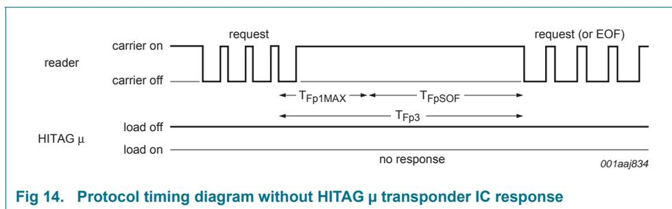
**Fig 14. Protocol timing diagram without HITAG  $\mu$  transponder IC response**
