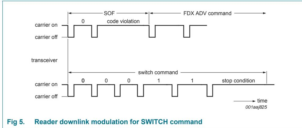
**Fig 5. Reader downlink modulation for SWITCH command**
