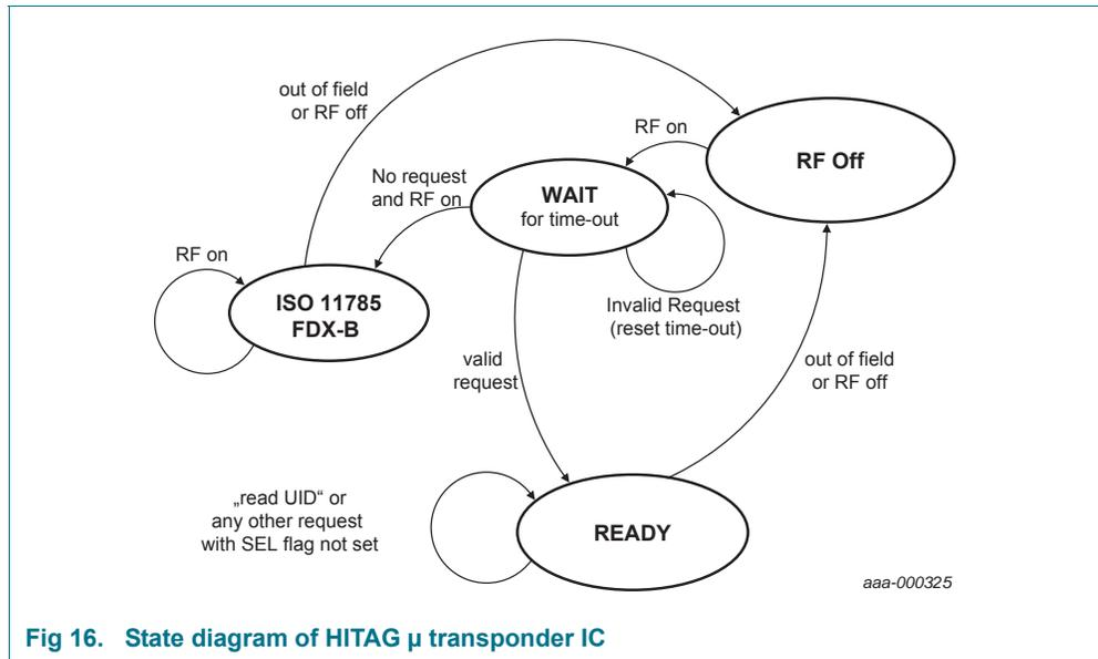
Fig 16. State diagram of HITAG  $\mu$  transponder IC
