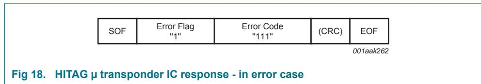
**Fig 18. HITAG μ transponder IC response - in error case**
