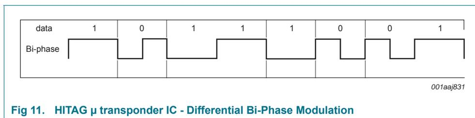
**Fig 11. HITAG  $\mu$  transponder IC - Differential Bi-Phase Modulation**
