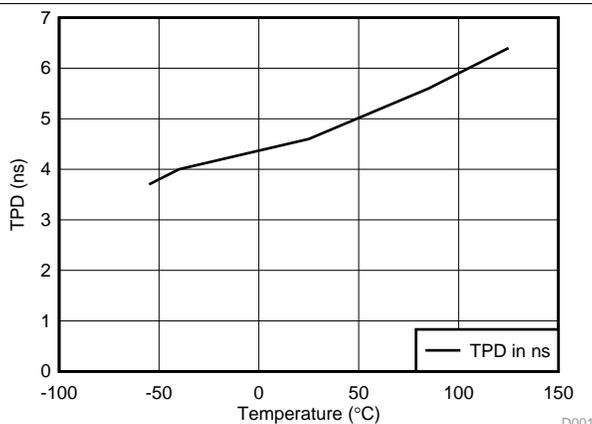
Figure 2. SN74AHCT595 TPD vs Temperature, 15 pF Load
