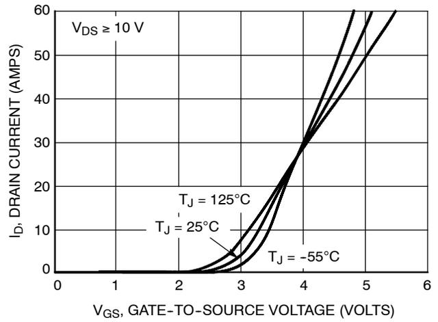
Figure 2. Transfer Characteristics
