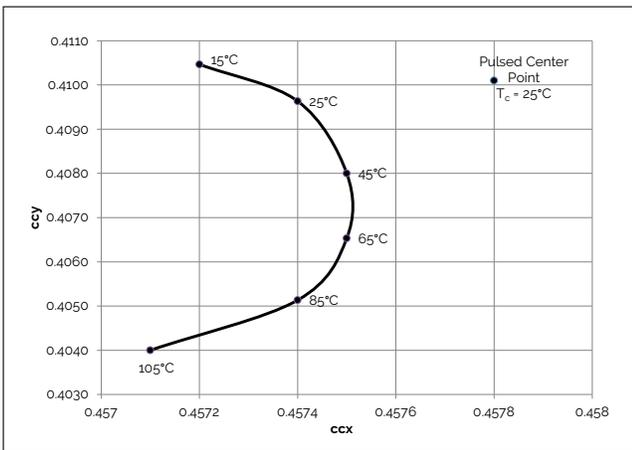
**Figure 12: 3000K, 90 CRI Color Shift vs. Case Temperature<sup>3</sup>**
