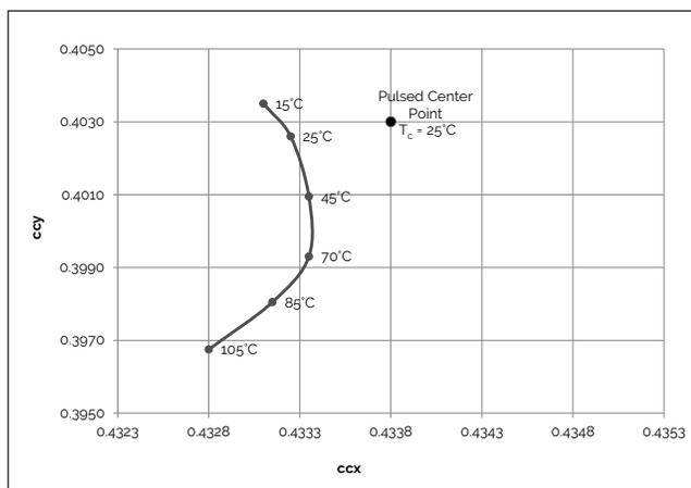
**Figure 14: 3500K Class A Color Shift vs. Case Temperature<sup>1</sup>**
