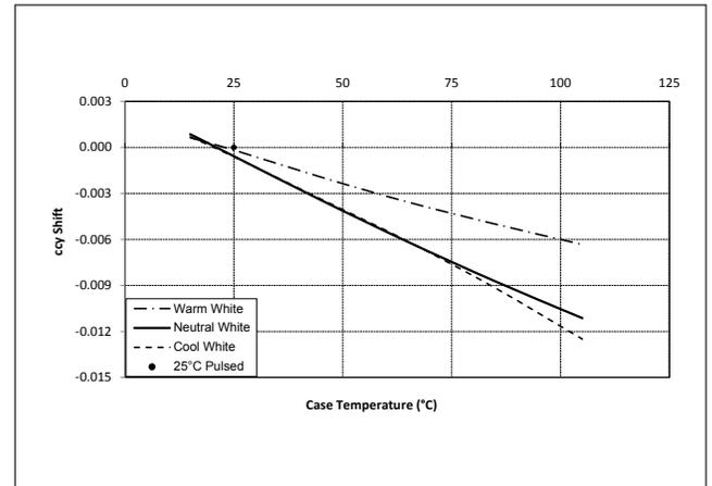
**Figure 7: Typical DC ccx Shift vs. Case Temperature**
