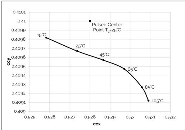
**Figure 10: 2500K Color Shift vs. Case Temperature<sup>1</sup>**
