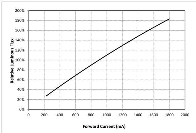
**Figure 4: V18C Typical Relative Flux vs. Current**
