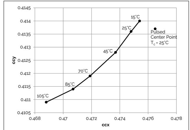
**Figure 11: 2700K, 97 CRI Color Shift vs. Case Temperature<sup>1</sup>**
