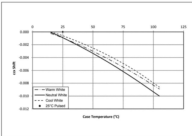
**Figure 8: 1750K Color Shift vs. Case Temperature<sup>1</sup>**
