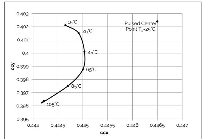
**Figure 13: 3000K, 97 CRI Color Shift vs. Case Temperature<sup>1</sup>**
