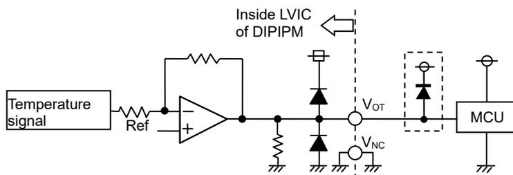
Fig.2-2-12  $V_{OT}$  output circuit in the case of using with low voltage controller
