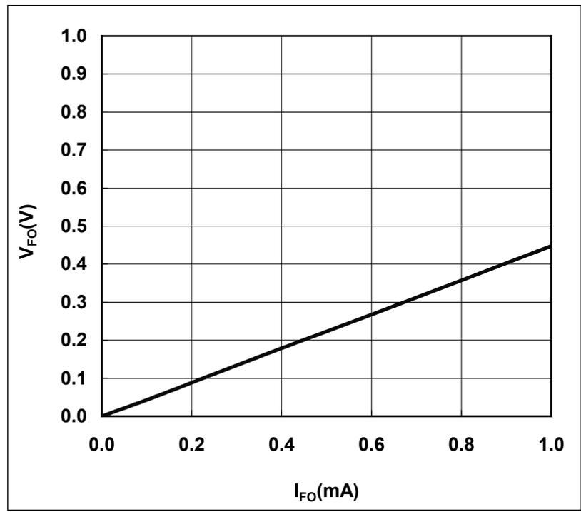
Fig.3-1-7 Fo terminal typical V-I characteristics (V<sub>D</sub>=15V, T<sub>J</sub>=25°C)
