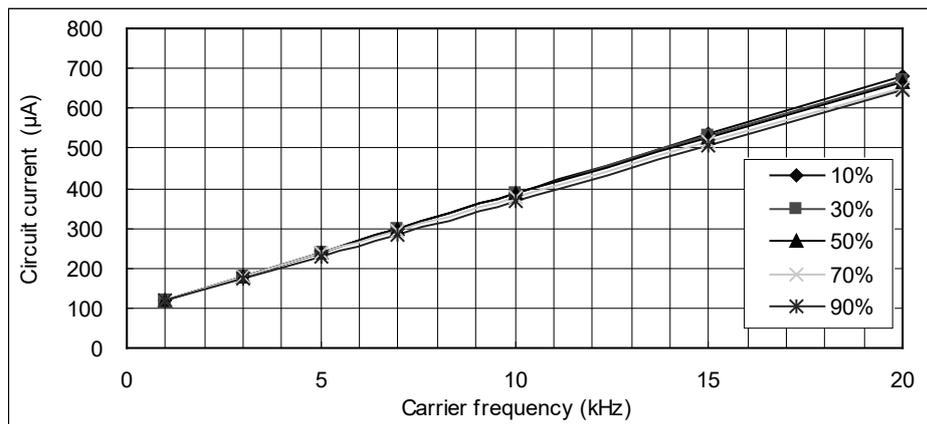
Fig.4-2-2  $I_{DB}$  vs. Carrier frequency for PSS10S92\*6-AG
