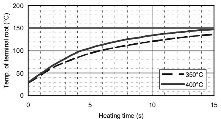
Fig.2-4-4 Temperature alteration of the terminal root (Example)
