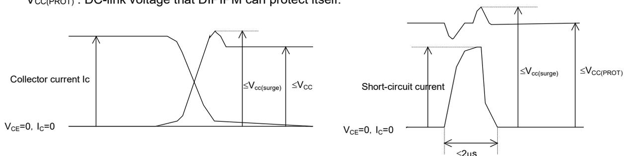
Fig.3-1-14 SOA at switching mode and short-circuit mode
