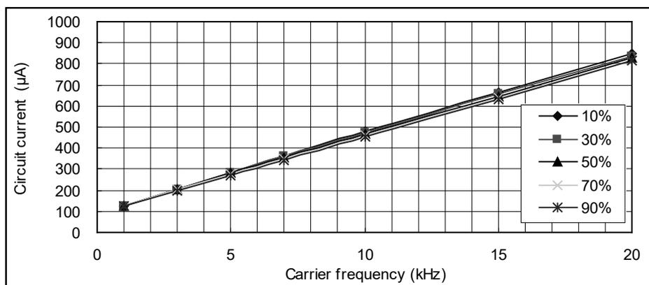
Fig.4-2-3  $I_{DB}$  vs. Carrier frequency for PSS15S92\*6-AG
