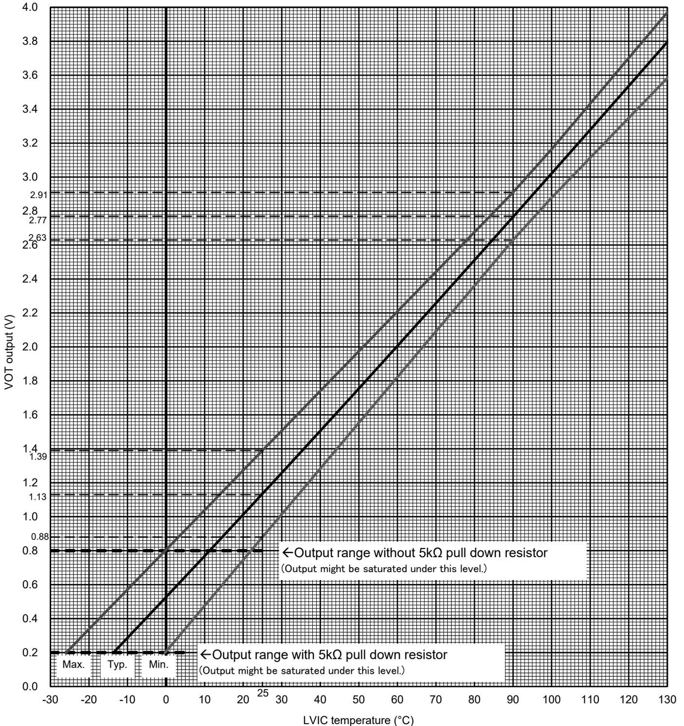
Fig.2-2-14 V<sub>OT</sub> output vs. LVIC temperature
