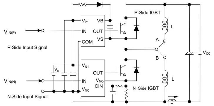
Fig.2-1-5 Evaluation circuit (inductive load)
