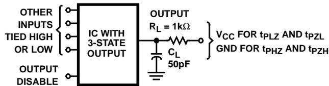
NOTE: Open-drain waveforms  $t_{PLZ}$  and  $t_{PZL}$  are the same as those for 3-state shown on the left. The test circuit is Output  $R_L = 1k\Omega$  to  $V_{CC}$ ,  $C_L = 50pF$ .
