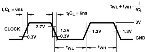
NOTE: Outputs should be switching from 10%  $V_{CC}$  to 90%  $V_{CC}$  in accordance with device truth table. For  $f_{MAX}$ , input duty cycle = 50%.
