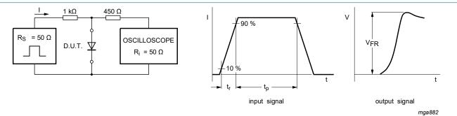
Input signal: forward pulse rise time  $t_r$  = 20 ns; forward current pulse duration  $t_p \ge 100$  ns; duty cycle  $\delta \le 0.005$
