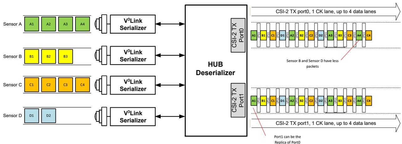
Figure 7-14. Four Sensor Data onto 1xCSI-2 Replicated With Virtual Channels (VC-ID) With Different Frame Size
