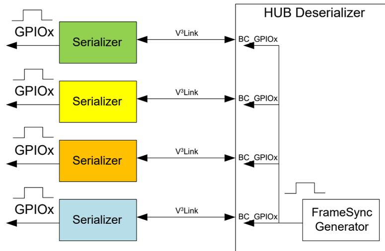
**Figure 7-16. Internal FrameSync**
