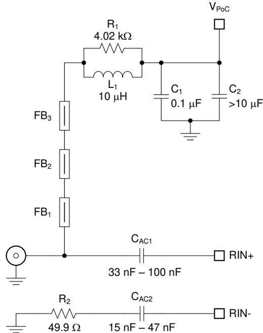
**Figure 8-2. Typical PoC Network for a "4G" V<sup>3</sup>Link**
