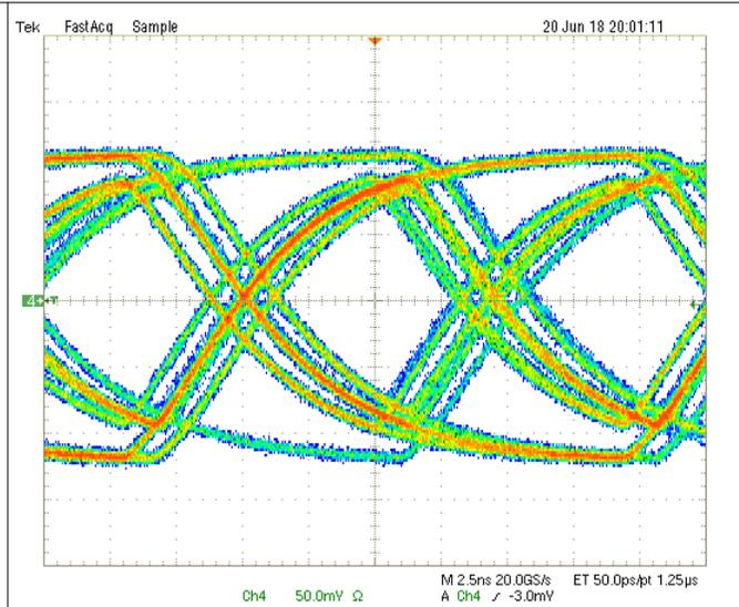
**Figure 6-12. Typical 50 Mbps Back Channel Output Waveform**
