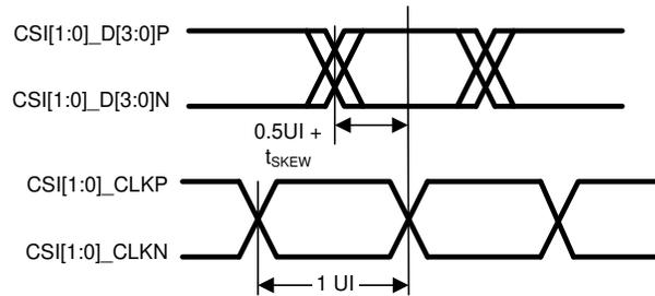
**Figure 6-5. Clock and Data Timing in HS Transmission**
