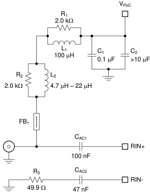
Figure 8-3. Typical PoC Network for a "2G" V<sup>3</sup>Link
