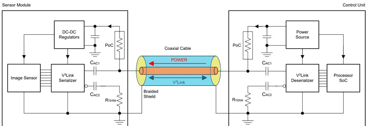
**Figure 8-1. Power-over-Coax (PoC) System Diagram**
