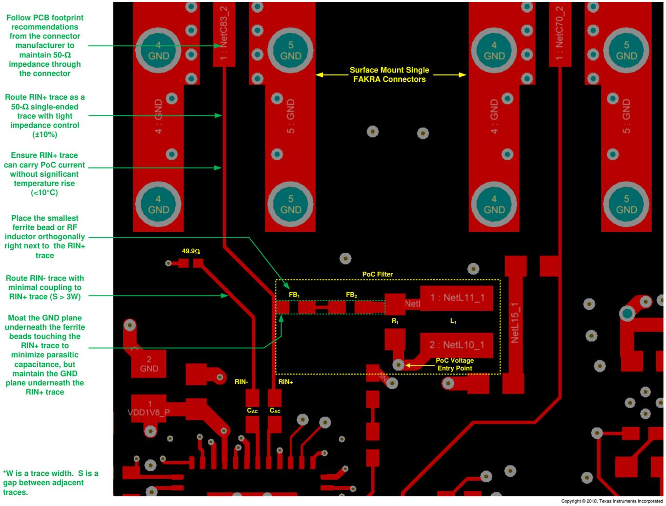
**Figure 10-2. Example Routing of V<sup>3</sup>Link Traces to a Single Mini-Fakra Connector and PoC Components**
