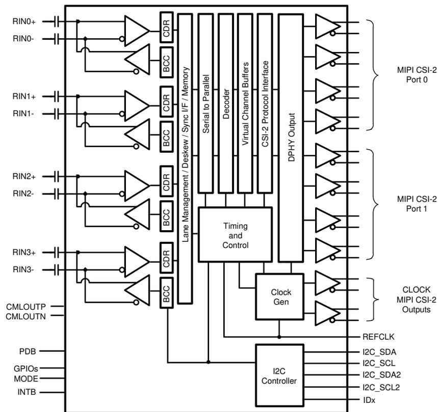
Figure 7-1. Functional Block Diagram
