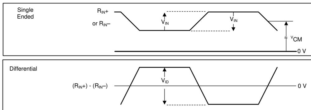
Figure 6-2. V<sup>3</sup>Link Receiver VID, VIN , VCM
