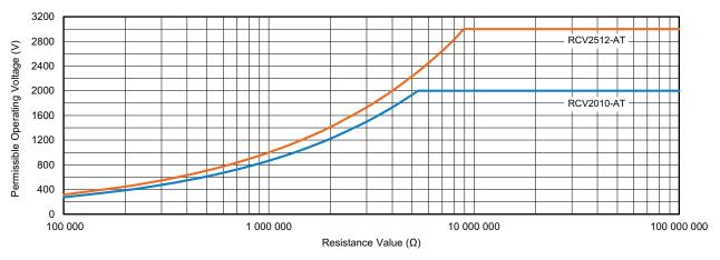
The permissible operating voltage  $U_{\text{max}}$  equals the rated voltage. For ambient temperatures above 70 °C power derating must be considered
