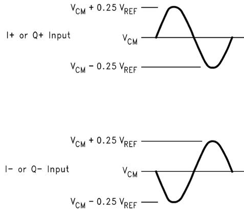
The ADC10D020 is designed for use with differential signals of 1.0 V<sub>P-P</sub> with a common mode voltage of 1.5V. The signal swing should not cause any pin to experience a swing more than 300 mV beyond the supply rails.
