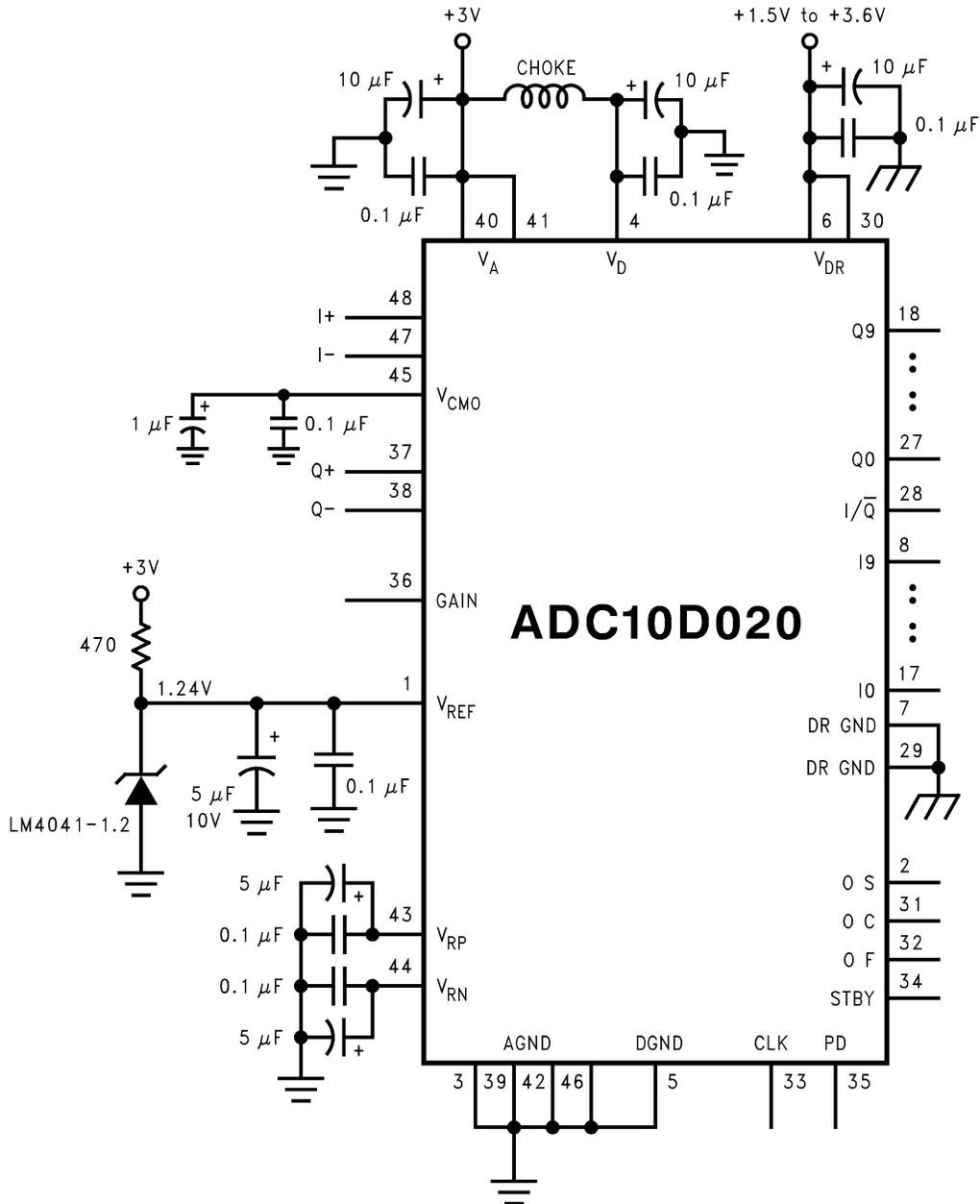
Figure 65. Improved Low Component Count Reference Biasing
