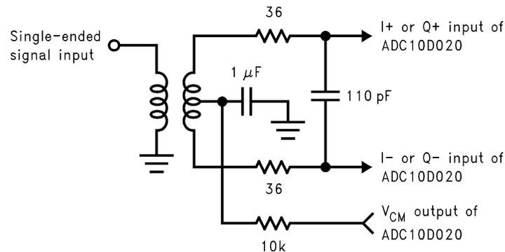
Use of an input transformer for single-ended to differential conversion can simplify circuit design for single-ended signals.
