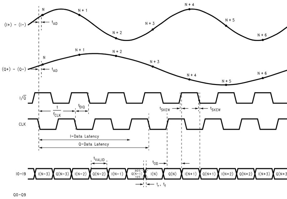
Figure 3. ADC10D020 Timing Diagram for Multiplexed Mode
