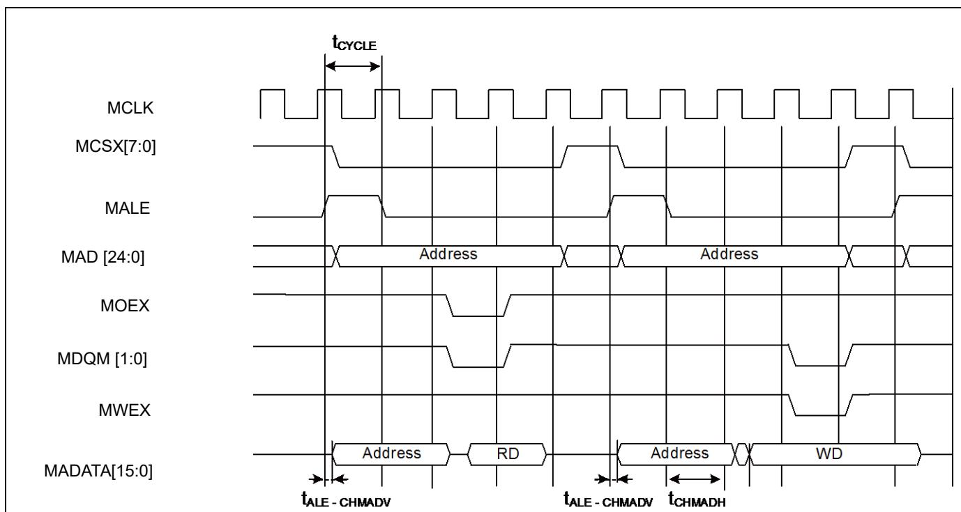
**Multiplexed Bus Access Synchronous SRAM Mode**
