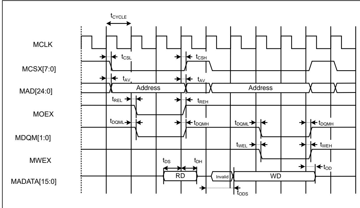
**Multiplexed Bus Access Asynchronous SRAM Mode**
