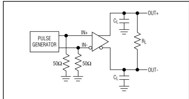
Figure 3. Transition Time and Propagation Delay Test Circuit
