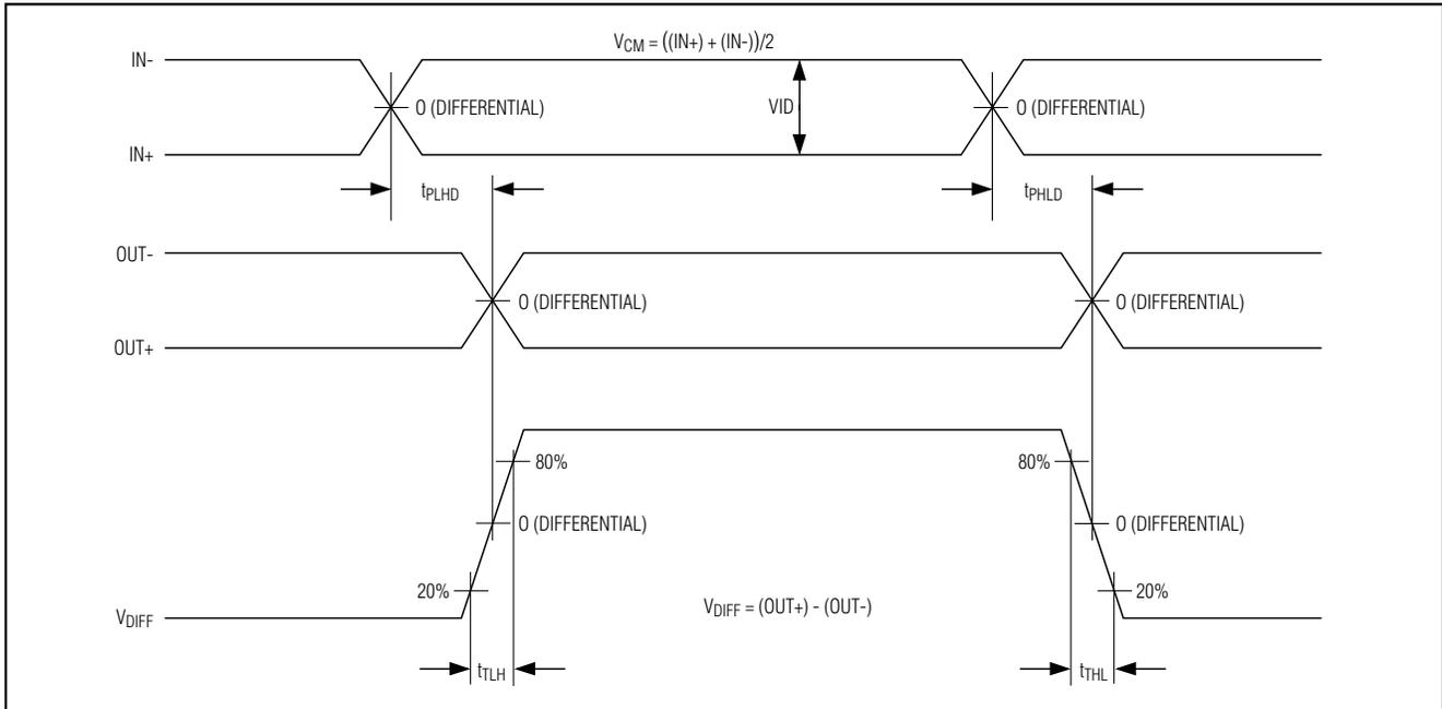
Figure 4. Transition Time and Propagation Delay Timing Diagram
