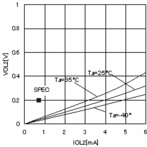
Figure 4. L output voltage  $V_{OL2-IOL2}$  ( $V_{CC}=1.7V$ )
