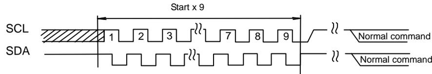
Figure 40-(c) START x 9 + command input
