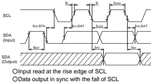
Figure 1-(a) Sync data input / output timing
