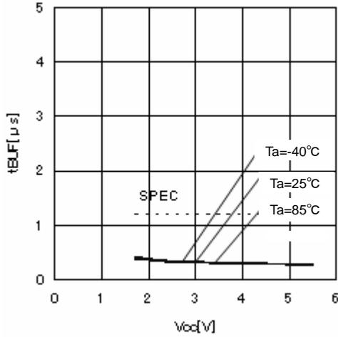
Figure 22. Bus release time before transfer start tBUF
