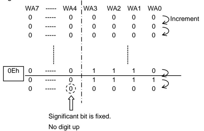
For example, when it is started from address 0Eh, therefore, increment is made as below, 0Eh→0Fh→00h→01h ---, which please note.
