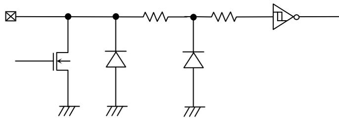
Figure 50. Input / output pin circuit diagram
