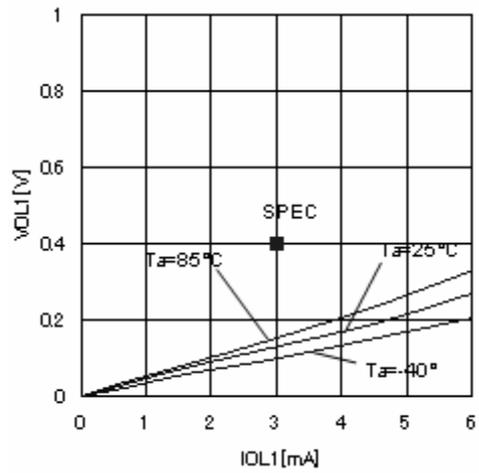
Figure 5. L input voltage  $V_{OL1-IOL1}$  ( $V_{CC}=2.5V$ )
