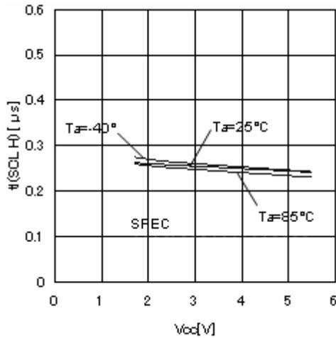
Figure 24. Noise removal time tI (SCL H)
