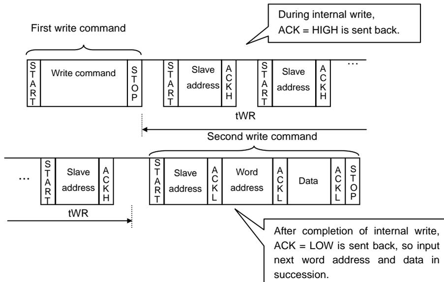
Figure 41. Case to continuously write by acknowledge polling
