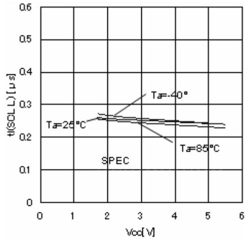
Figure 25. Noise removal time tI (SCL L)
