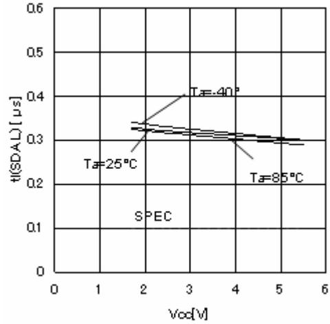
Figure 27. Noise removal time  $t_I$  (SDA L)
