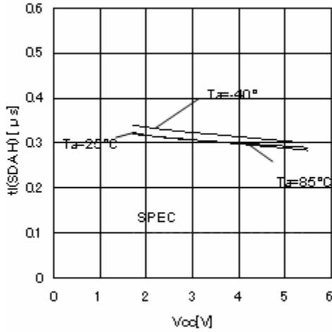
Figure 26. Noise removal time  $t_I$  (SDA H)
