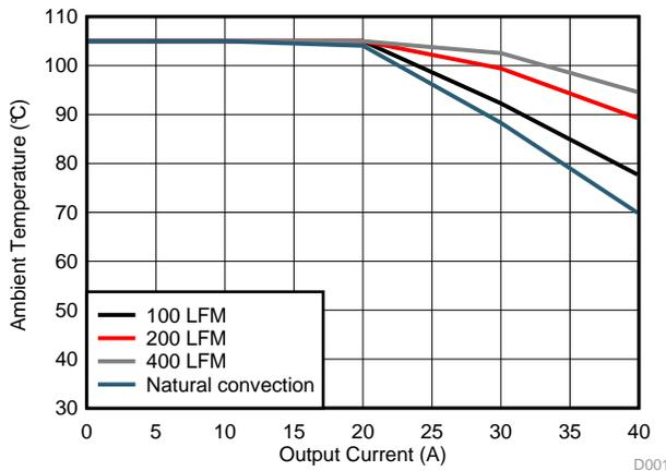
$V_{IN} = 12\text{ V}$       $V_{OUT} = 1\text{ V}$       $f_{SW} = 650\text{ kHz}$
