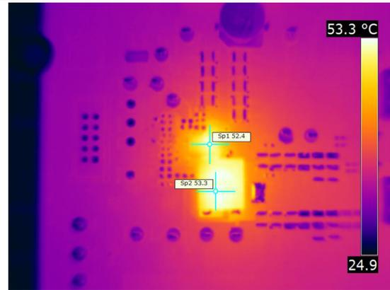
$V_{IN} = 12\text{ V}$        $f_{SW} = 425\text{ kHz}$        $I_{OUT} = 30\text{ A}$
