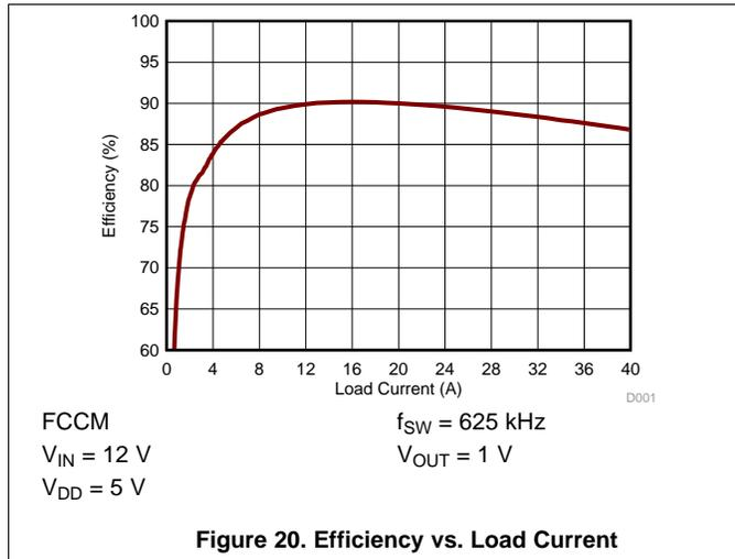
Figure 20. Efficiency vs. Load Current
