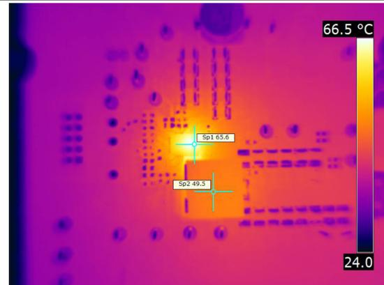
$V_{IN} = 12\text{ V}$        $f_{SW} = 650\text{ kHz}$        $I_{OUT} = 40\text{ A}$
