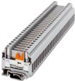
Disconnect terminal block, Connection method: Screw connection, Cross section: 0.5 mm<sup>2</sup> - 16 mm<sup>2</sup>, AWG: 20 - 8, Width: 10.2 mm, Mounting type: NS 35/7,5, NS 35/15, NS 32, Color: gray
