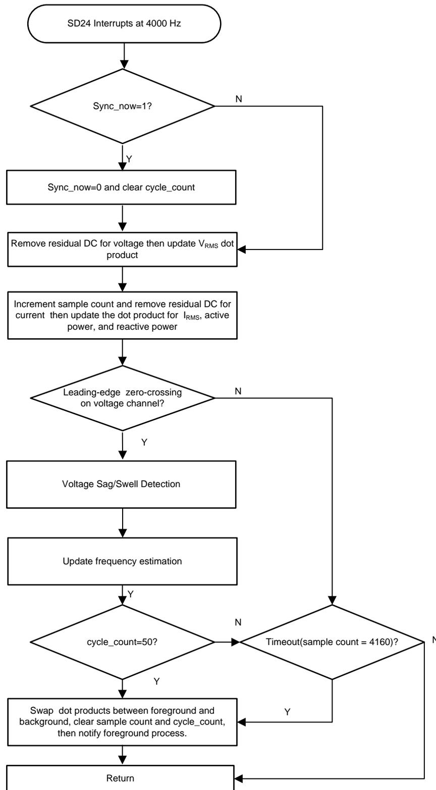
**Figure 10. per\_sample\_dsp Function**
