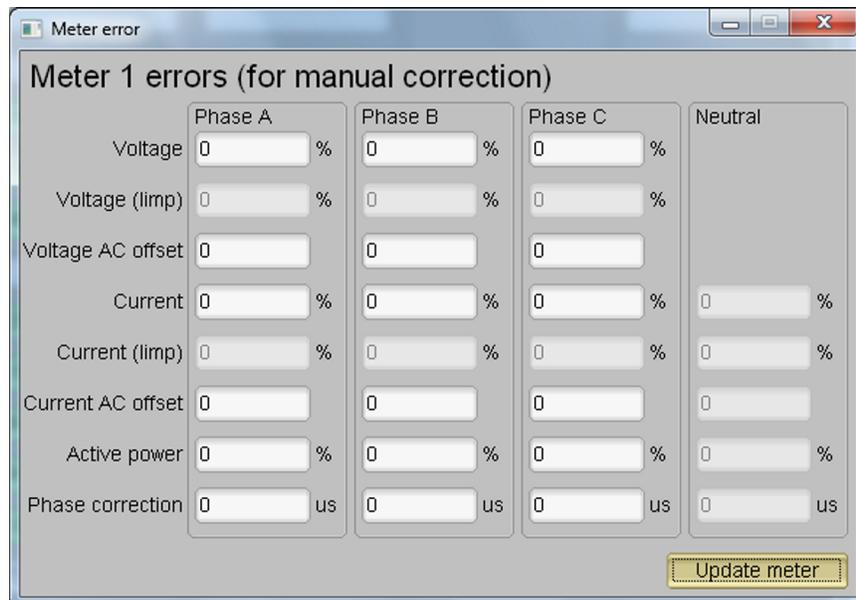
**Figure 34. Manual Calibration Window**
