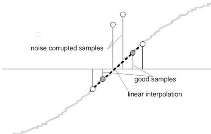
**Figure 11. Frequency Measurement**
