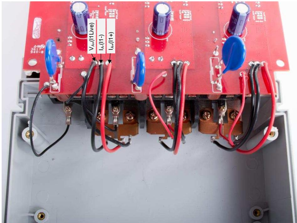
**Figure 19. Mapping Between Shunt Terminals and Ix Current Pads**
