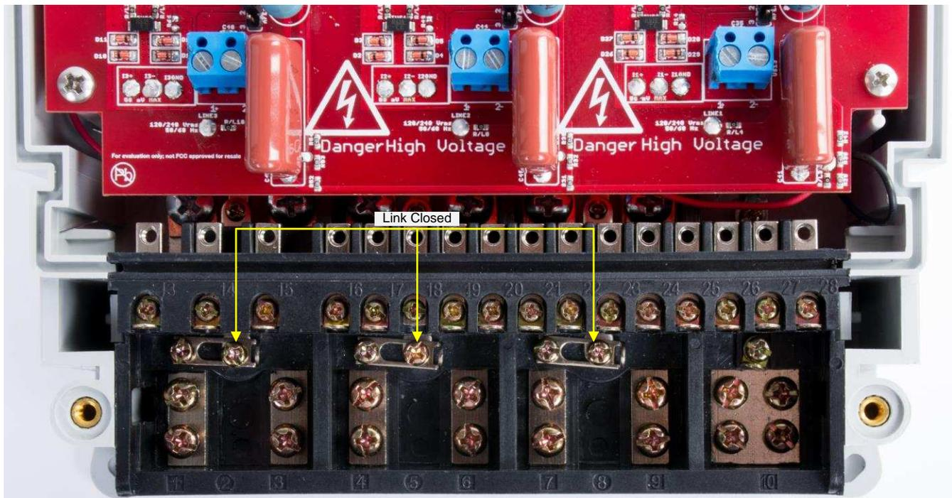
**Figure 20. Top View of EVM With Links Closed**
