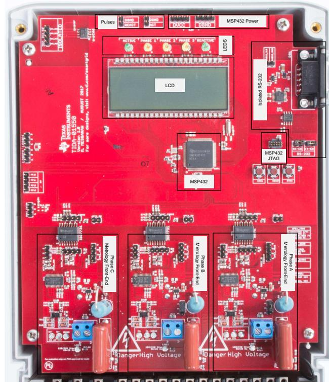
Figure 18. Top View of Reference Design With Components Highlighted
