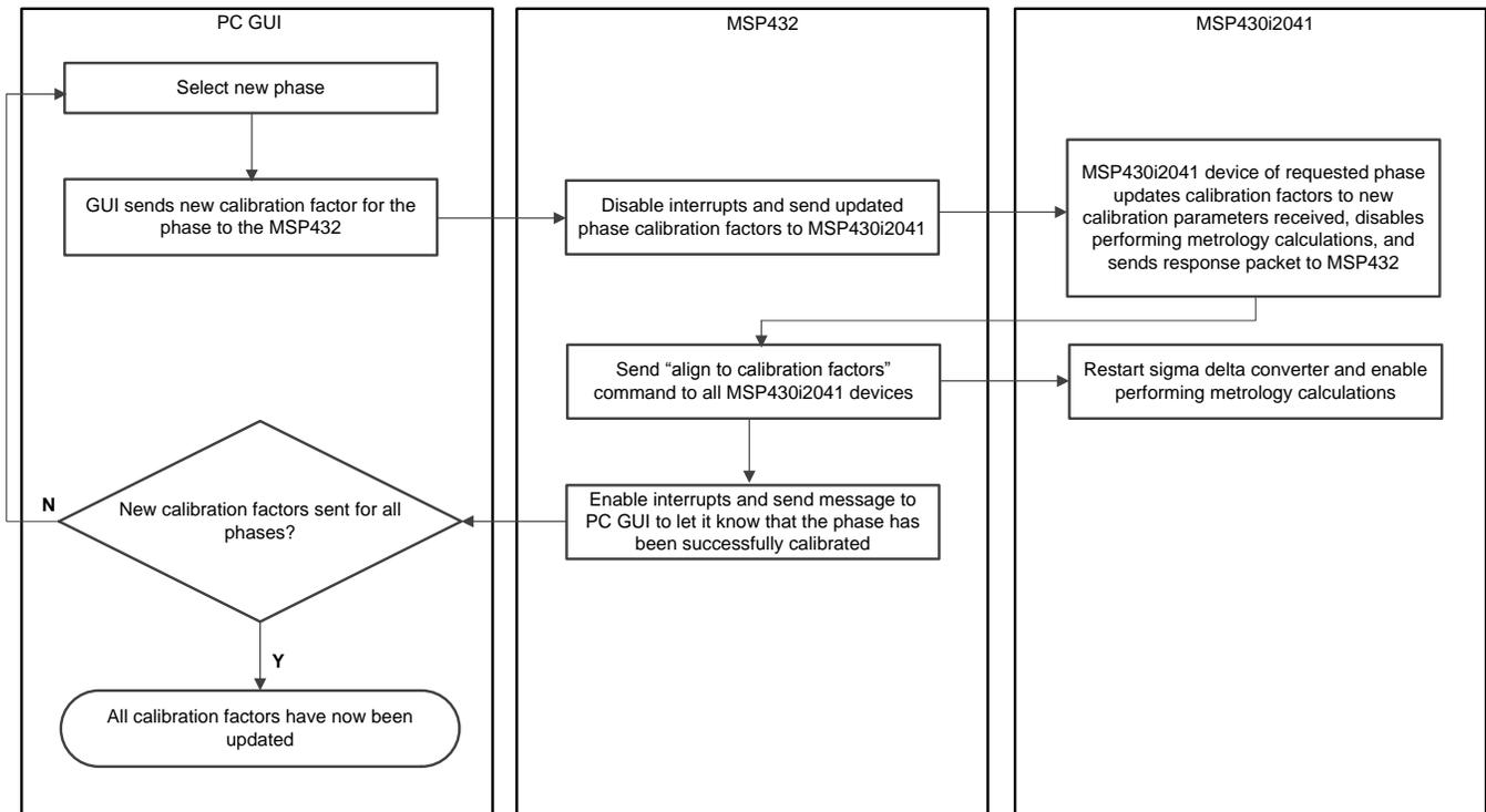
**Figure 16. Process for Setting New Calibration Factors**
