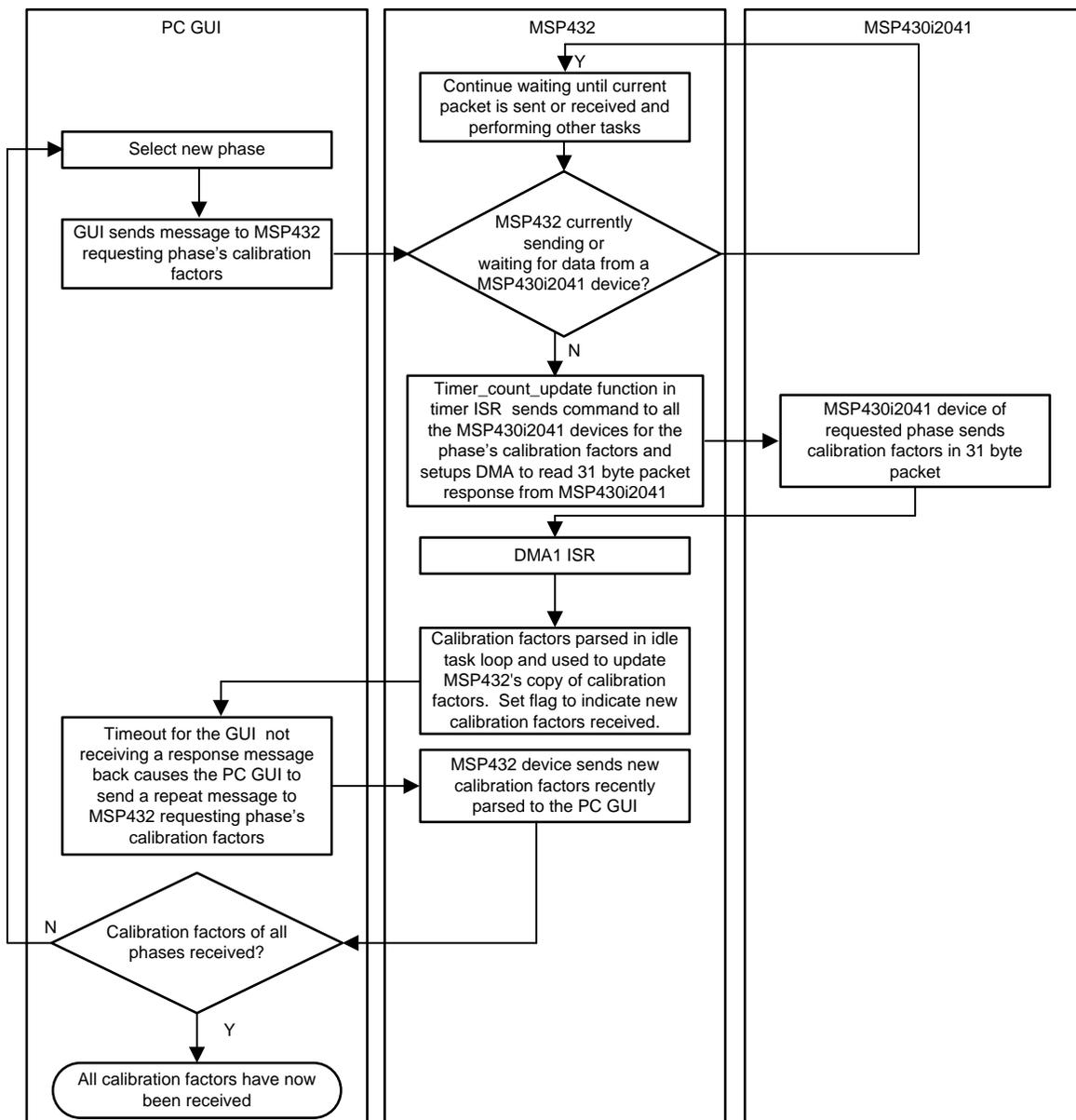
Figure 15. Process for Obtaining All Calibration Factors
