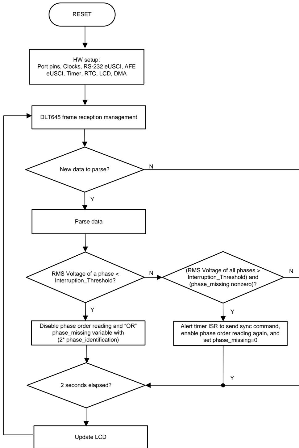
**Figure 12. Peripheral Setup and Idle Tasks**
