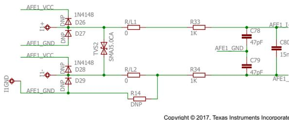
Figure 7. MSP430i2041 Current Front-End Circuitry
