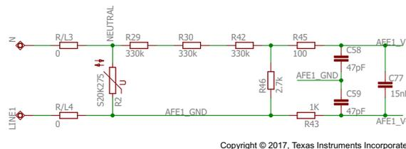
Figure 6. MSP430i2041 Voltage Front-End Circuitry
