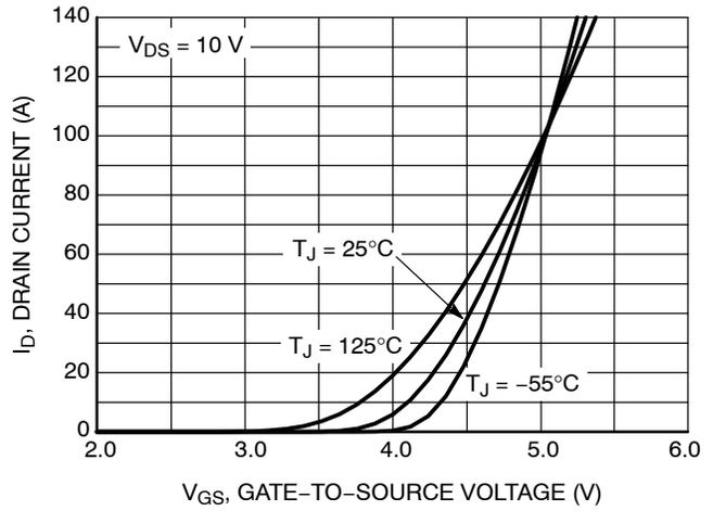
Figure 2. Transfer Characteristics
