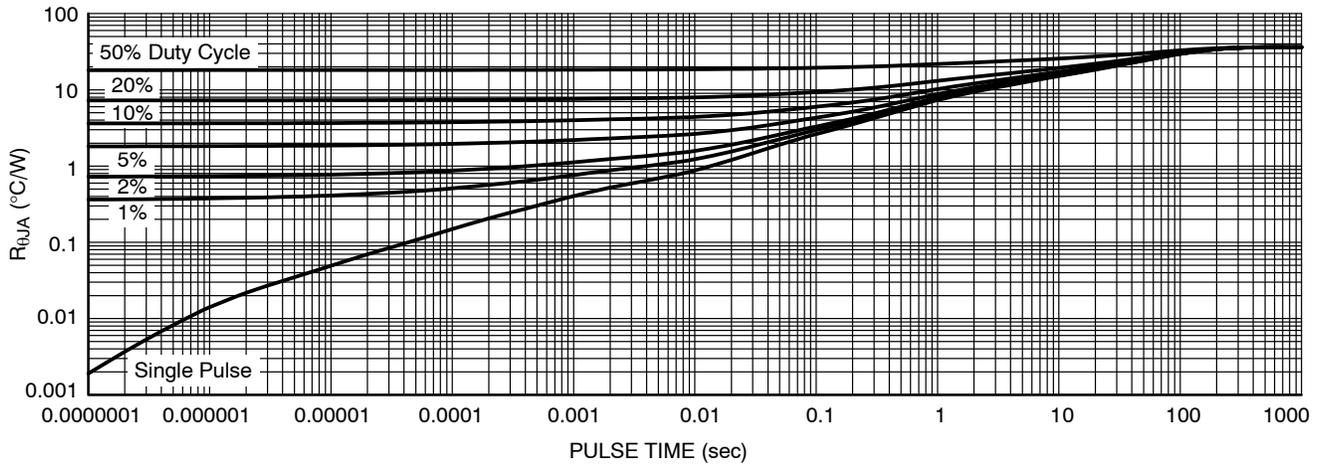
Figure 13. Thermal Characteristics
