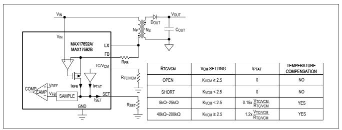
Figure 7. TC/V<sub>CM</sub> Pin Configuration
