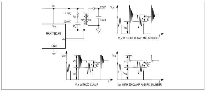
Figure 9. Voltage Clamp Circuit
