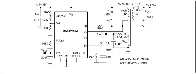
Figure 10. 24V to 5V, 0.65A MAX17692B No-Opto Flyback Application Circuit
