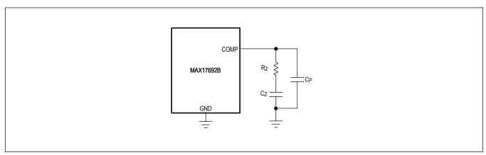
Figure 8. MAX17692B Loop Compensation Arrangement
