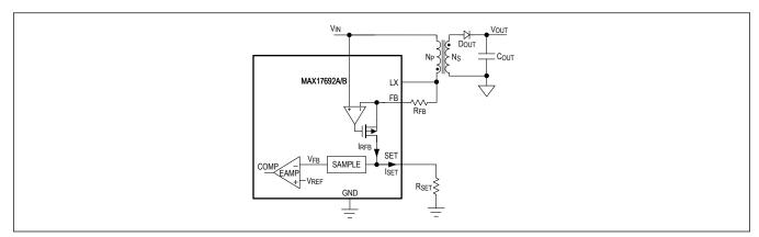
Figure 6. Simplified diagram of No-Opto Flyback Operation
