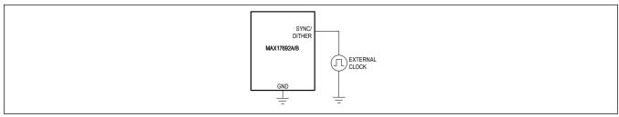
Figure 5. External Clock Synchronization Configuration
