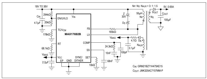
Figure 11. 24V to 5V, 0.65A MAX17692B No-Opto Flyback Application Circuit
