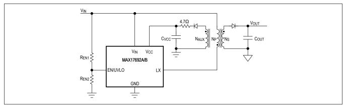
Figure 1. V<sub>CC</sub> Pin Overdrive Configuration
