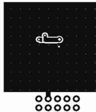
a. 50  $^\circ\text{C}/\text{W}$  when mounted on a 1 in<sup>2</sup> pad of 2 oz copper.
