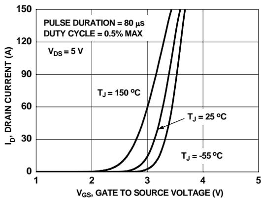
Figure 5. Transfer Characteristics
