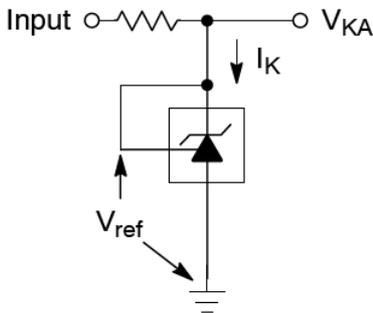
**Figure 1:  $V_{KA} = V_{REF}$**
