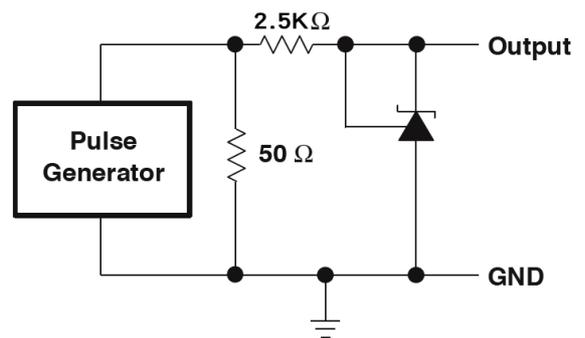
Test Circuit for Pulse Response,  $I_{k1} = 1mA$
