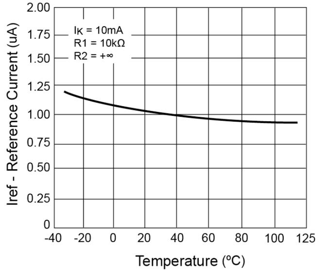
Figure 20: Reference Current vs. Temperature
