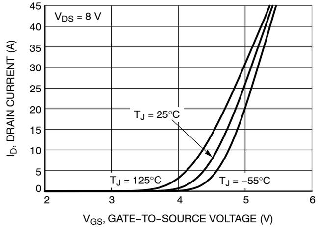
Figure 2. Transfer Characteristics
