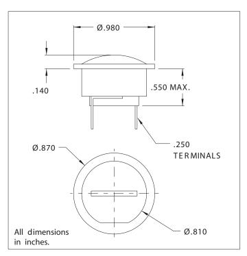
Mounting: Supplied with speednut SN2089. Mounting hole pattern on page SP2.
