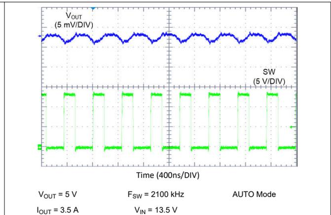
Figure 9-18. LM62435-Q1 Switching Waveform and  $V_{OUT}$  Ripple
