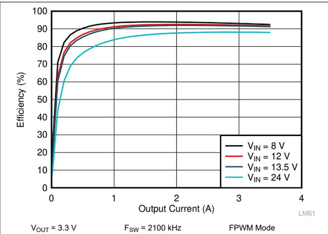
**Figure 9-6. LM62435-Q1 Efficiency**
