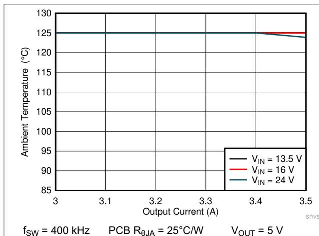
**Figure 9-2. Maximum Ambient Temperature versus Output Current**
