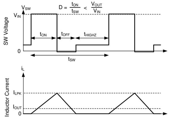
In auto mode, the low-side device is turned off once SW node current is near zero. As a result, once output current is less than half of what inductor ripple would be in CCM, the part operates in DCM which is equivalent to the statement that diode emulation is active.
