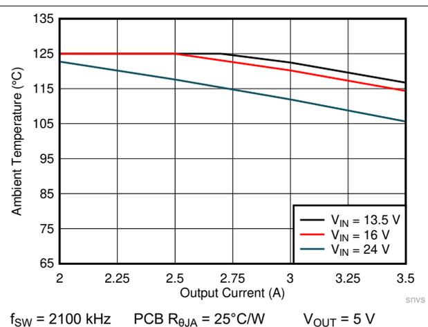
**Figure 9-3. Maximum Ambient Temperature versus Output Current**
