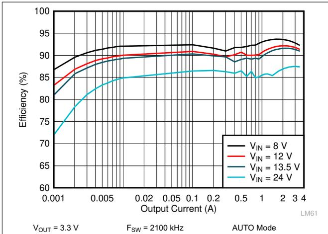
**Figure 9-5. LM62435-Q1 Efficiency**
