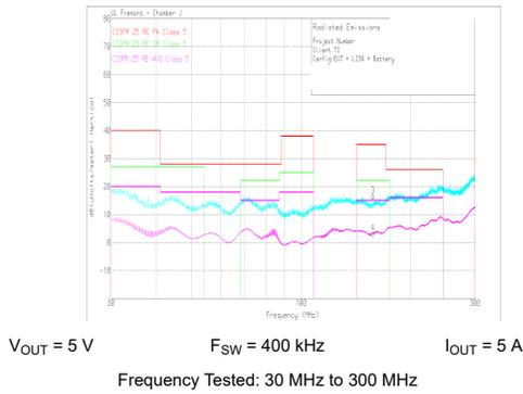
**Figure 9-29. Radiated EMI Bicon Horizontal versus CISPR25 Limits**
