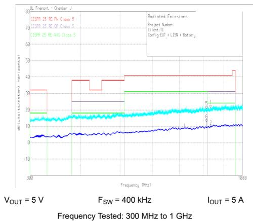
**Figure 9-31. Radiated EMI Log Horizontal versus CISPR25 Limits**
