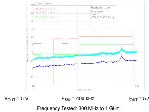
**Figure 9-30. Radiated EMI Log Vertical versus CISPR25 Limits**
