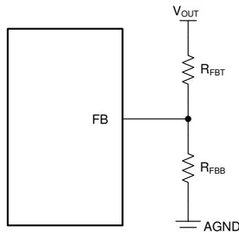
**Figure 8-17. Setting Output Voltage of Adjustable Versions**
