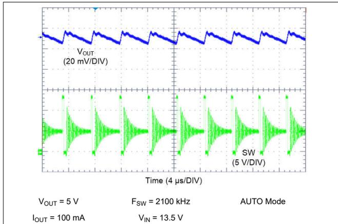
Figure 9-17. LM62435-Q1 Switching Waveform and  $V_{OUT}$  Ripple
