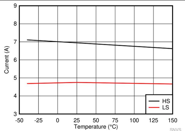
**Figure 7-4. LM62435-Q1 High-side and Low-side Current Limits**
