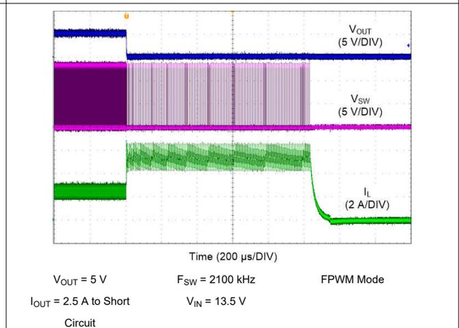
Figure 9-20. LM62435-Q1 Short Circuit Protection
