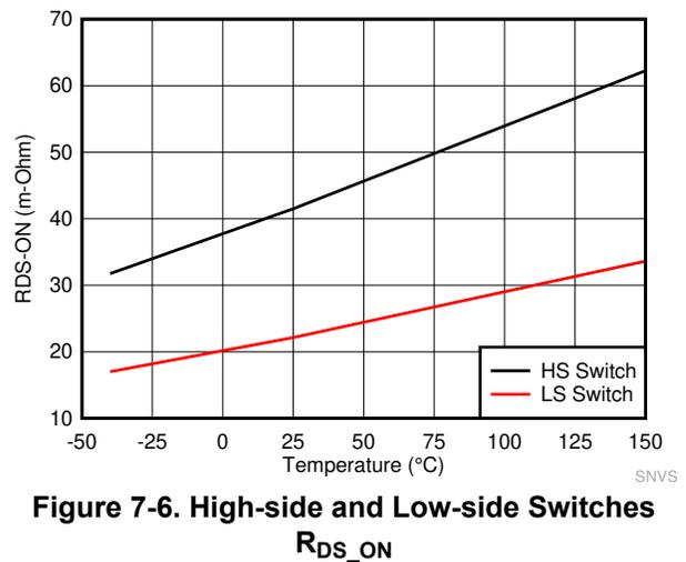
**Figure 7-6. High-side and Low-side Switches  $R_{DS\_ON}$**
