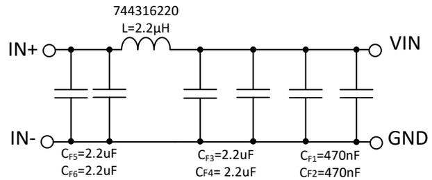
$F_{SW} = 400\text{ kHz}$       Note: Measurements taken with LM61460EVM with 6 A variant
