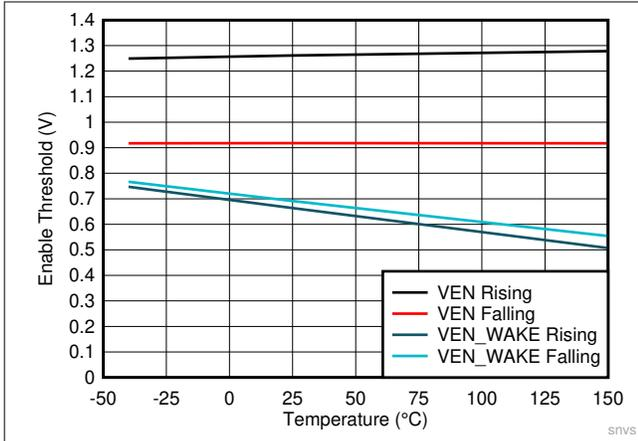
Figure 7-7. Enable Thresholds
