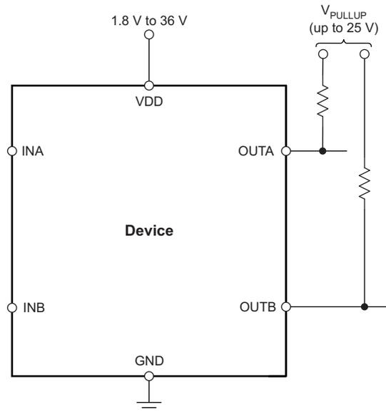
**Figure 21. Interfacing to Voltages Other than  $V_{DD}$**
