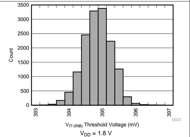
Figure 11. INB Negative Input Threshold Voltage ( $V_{IT-(INB)}$ ) Distribution
