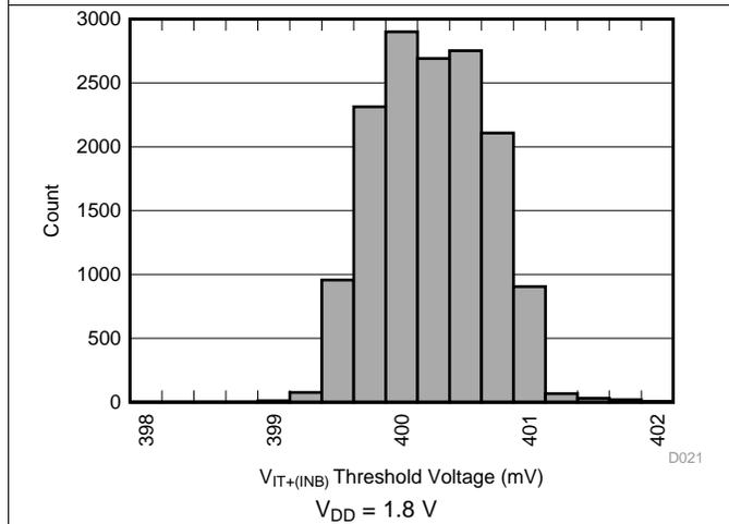
Figure 10. INB Positive Input Threshold Voltage ( $V_{IT+(INB)}$ ) Distribution
