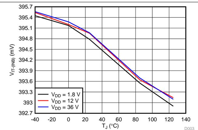
Figure 7. INB Negative Input Threshold Voltage ( $V_{IT-(INB)}$ ) vs Temperature
