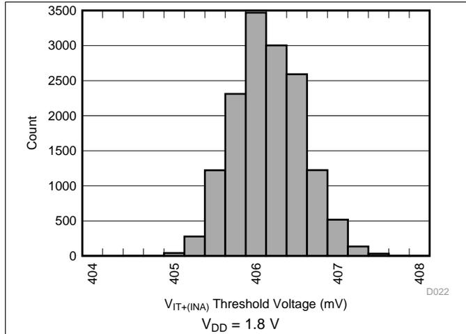
Figure 8. INA Positive Input Threshold Voltage ( $V_{IT+(INA)}$ ) Distribution
