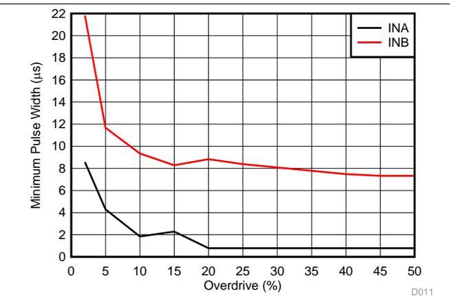
Figure 3. Minimum Pulse Duration vs Threshold Overdrive Voltage<sup>(1)</sup> (1)
