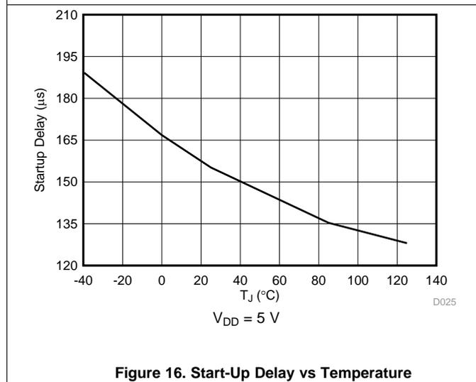
Figure 16. Start-Up Delay vs Temperature
