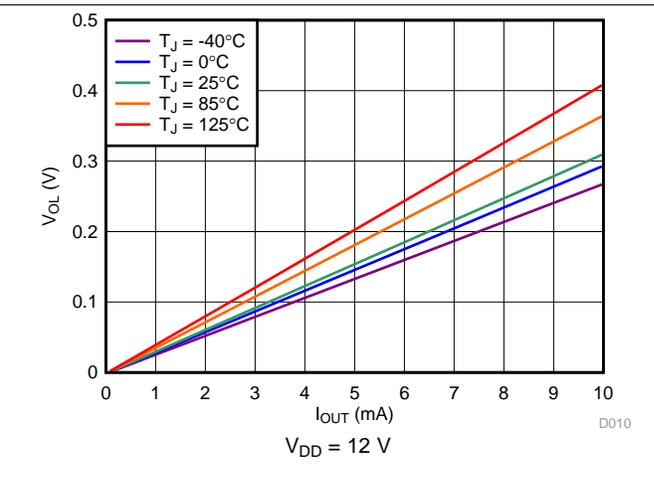
Figure 15. Output Voltage Low vs Output Sink Current
