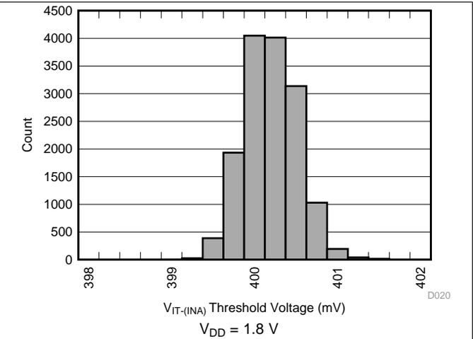
Figure 9. INA Negative Input Threshold Voltage ( $V_{IT-(INA)}$ ) Distribution
