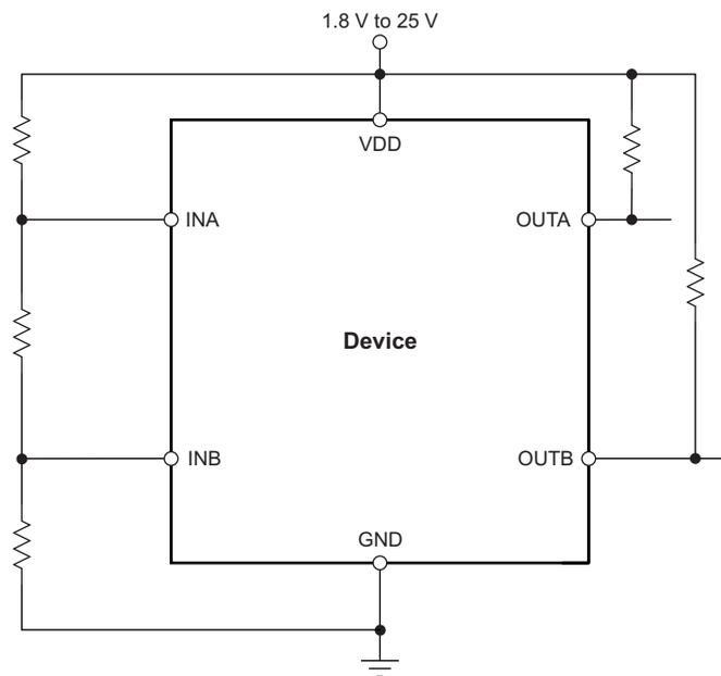
**Figure 22. Monitoring the Same Voltage as  $V_{DD}$**
