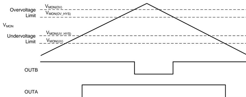
Figure 20. Window Comparator Timing Diagram
