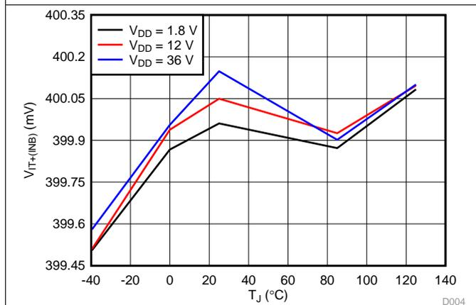
Figure 6. INB Positive Input Threshold Voltage ( $V_{IT+(INB)}$ ) vs Temperature
