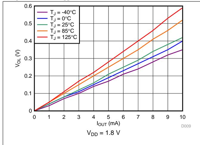
Figure 14. Output Voltage Low vs Output Sink Current
