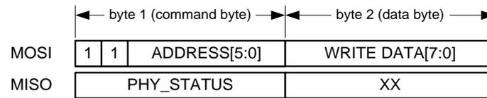
Each register access must be terminated by setting /SEL = H.
