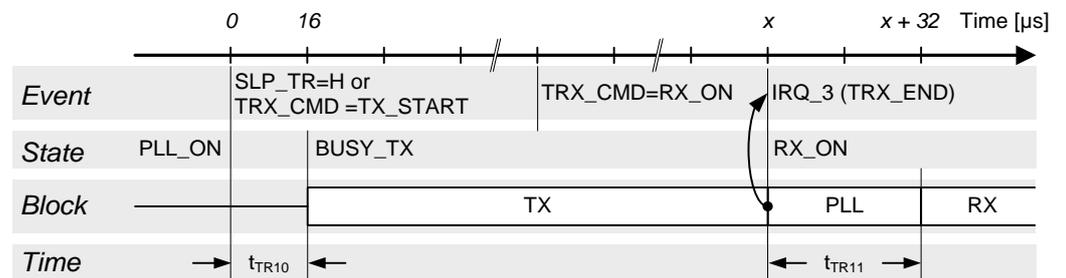
Starting from PLL\_ON state, it is further assumed that the PLL has already been locked. A transmission is initiated either by a rising edge of pin 11 (SLP\_TR) or by command TX\_START. The PLL settles to the transmit frequency and the PA is enabled. After the duration of  $t_{TR10}$  (one symbol period), the Atmel AT86RF212B
