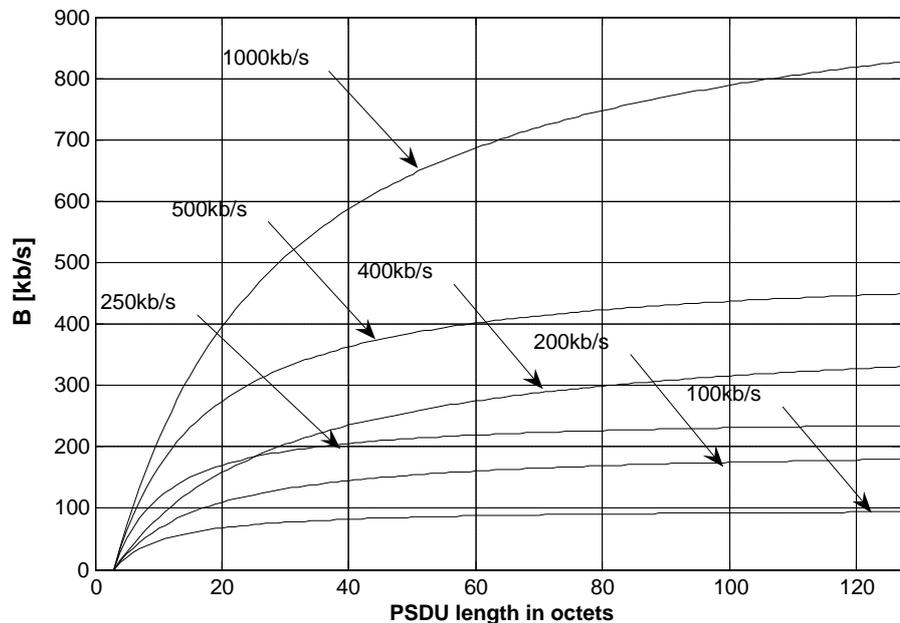
Consequently, high data rate transmission is useful for large PSDU lengths due to the higher effective data rate, or in order to reduce the power consumption of the system.
