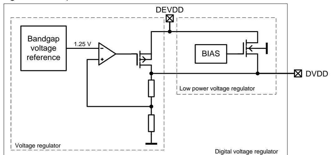
The block “Low power voltage regulator” within the “Digital voltage regulator” maintains the DVDD supply voltage at 1.5V (typical) when the Atmel AT86RF212B voltage regulator is disabled in sleep mode. All configuration register values are stored.
