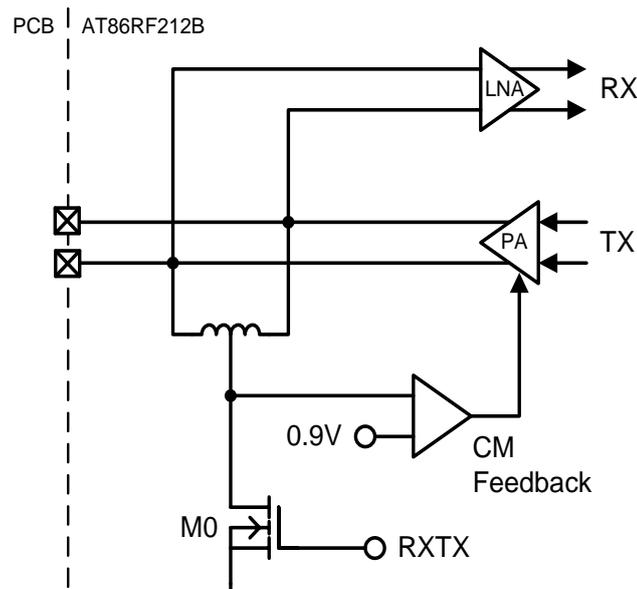
The RF port DC values depend on the operating state; refer to [Chapter 7](#). In TRX\_OFF state, when the analog front-end is disabled (see [Section 7.1.2.3](#)), the RF pins are pulled to ground, preventing a floating voltage larger than 1.8V which is not allowed for the internal circuitry.
