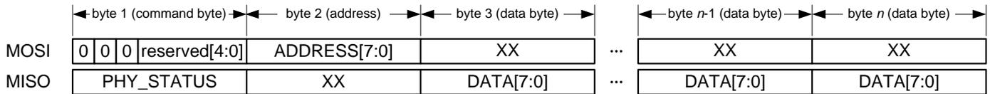
On SRAM write access, one or more bytes of write data are transferred on MOSI starting with the third byte of the access sequence; refer to [Figure 6-12](#). Do not attempt to read or write bytes beyond the SRAM buffer size.
