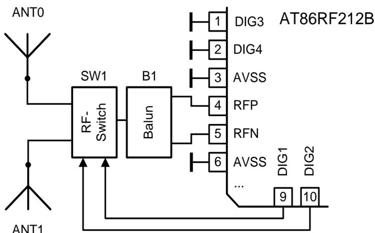
Generally, when the external RF-Switch (SW1) is to be controlled by antenna diversity algorithm, the antenna diversity enable must be activated by register bit ANT\_EXT\_SW\_EN (register 0x0D, ANT\_DIV). Then the digital control pins pin 9 (DIG1) and pin 10 (DIG2) are enabled (refer to [Section 1.3](#)) to drive the antenna switch control signals to the differential inputs of the RF Switch (SW1) to switch between ANT0 and ANT1.
