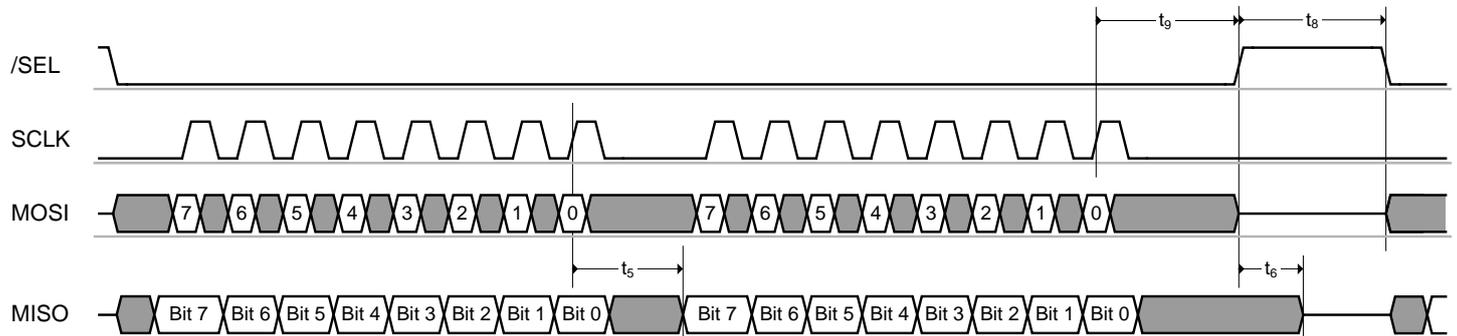
**Figure 6-3.** SPI Timing, Detailed Drawing of Timing Parameters  $t_1$  to  $t_4$ .
