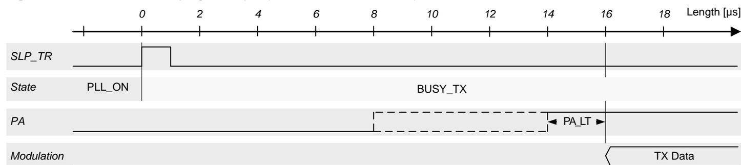
Using an external RF front-end (refer to Section 11.4), it may be required to adjust the startup time of the external PA relative to the internal building blocks to optimize the overall PSD. This can be achieved using register bits PA\_LT (register 0x16, RF\_CTRL\_0).
