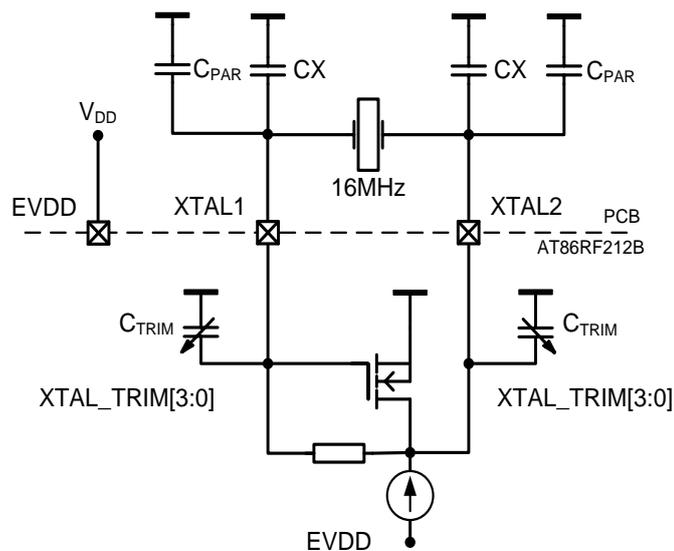
Additional internal trimming capacitors  $C_{TRIM}$  are available. Any value in the range from 0pF to 4.5pF with a 0.3pF resolution is selectable using XTAL\_TRIM of register 0x12 (XOSC\_CTRL). To calculate the total load capacitance, the following formula can be used
