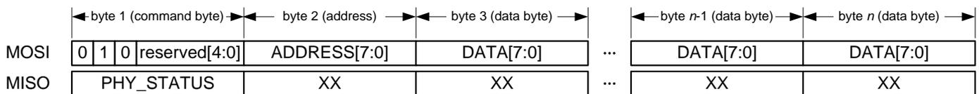
As long as /SEL = L, every subsequent byte read or byte write increments the address counter of the Frame Buffer until the SRAM access is terminated by /SEL = H.
