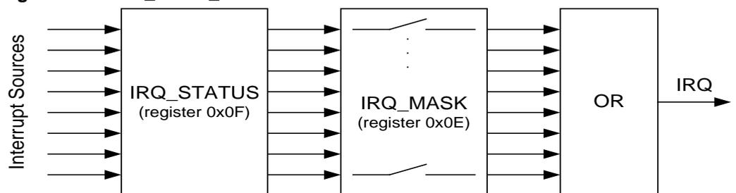
The Atmel AT86RF212B IRQ pin polarity can be configured with register bit `IRQ_POLARITY` (register `0x04`, `TRX_CTRL_1`). The default behavior is active high, which means that pin 24 (IRQ) = H issues an interrupt request.
