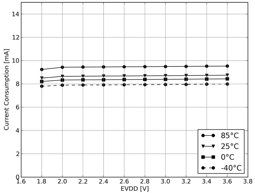
Figure 13-6. Current Consumption in RX\_ON State – Reduced Sensitivity.
