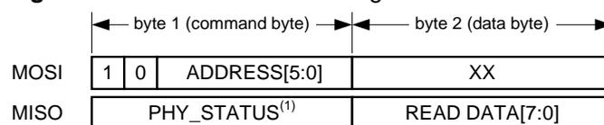
Note: 1. Each SPI access can be configured to return radio controller status information (PHY\_STATUS) on MISO, for details refer to [Section 6.4](#).
