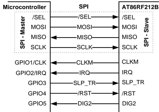
Microcontrollers with a master SPI such as Atmel AVR family interface directly to the AT86RF212B. The SPI is used for register, Frame Buffer, SRAM, and AES access. The additional control signals are connected to the GPIO/IRQ interface of the microcontroller. [Table 6-1](#) introduces the radio transceiver I/O signals and their functionality.
