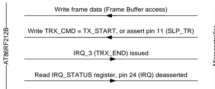
Alternatively for time critical applications when the frame start transmission time needs to be minimized, a frame transmission task can be started first. Then it can be followed by the Frame Buffer write access event (populating PSDU data). This way the data to be transmitted is needs to be written in the transmit frame buffer as the transceiver initializes and begins SHR transmission; refer to Figure 10-3.
