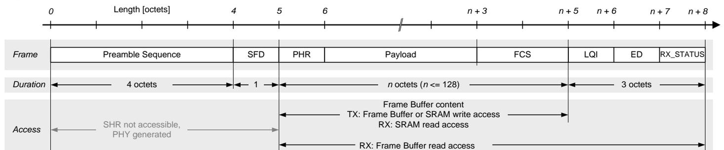
A frame comprises two sections, the radio transceiver internally generated SHR field and the user accessible part stored in the Frame Buffer. The SHR contains the preamble and the SFD field. The variable frame section contains the PHR and the PSDU including the FCS, see [Section 8.3](#).
