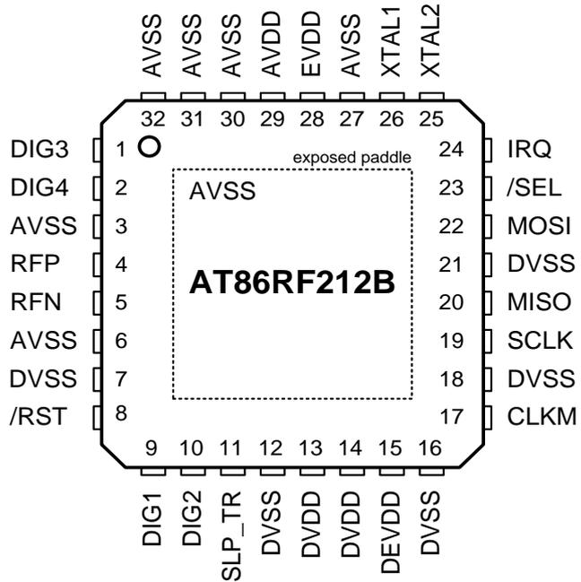
Note: 1. The exposed paddle is electrically connected to the die inside the package. It shall be soldered to the board to ensure electrical and thermal contact and good mechanical stability.
