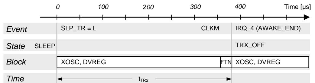
The radio transceiver's SLEEP state is left by releasing pin 11 (SLP\_TR) to logic low. This restarts the XOSC and DVREG. After  $t_{TR2} = 420\mu s$  (typ.) the radio transceiver enters TRX\_OFF state. The internal clock signal is available and provided to pin 17 (CLKM), if enabled.
