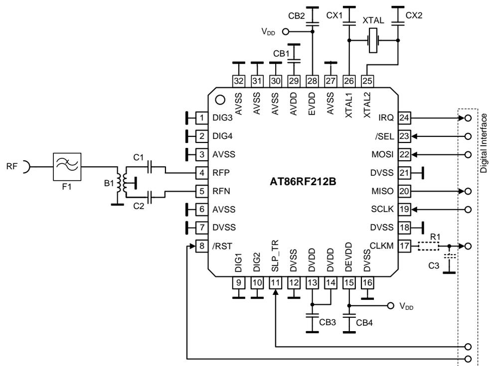
The power supply decoupling capacitors (CB2, CB4) are connected to the external analog supply pin 28 (EVDD) and external digital supply pin 15 (DEVDD). Capacitors CB1 and CB3 are bypass capacitors for the integrated analog and digital voltage regulators to ensure stable operation. All bypass capacitors should be placed as close as possible to the pins and should have a low-resistance and low-inductance connection to ground to achieve the best performance.
