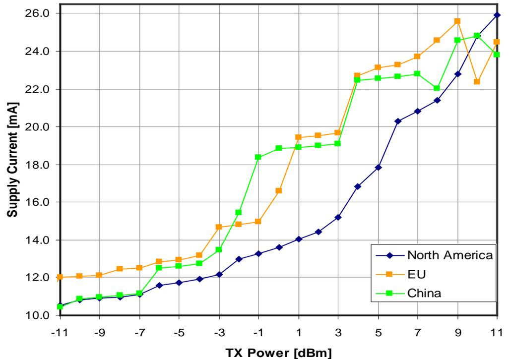
The North American mapping table is optimized for lowest supply current. The more relaxed spectral side lobe requirements of the IEEE 802.15.4 standard are fulfilled.
