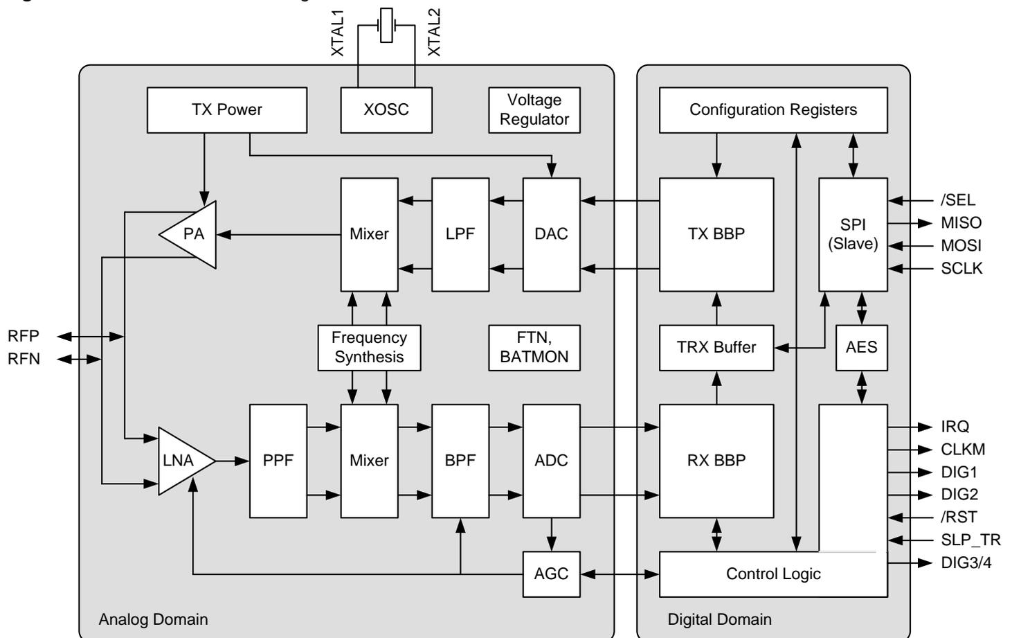
The number of external components is minimized so that only the antenna, a filter (at high output power levels), the crystal, and four bypass capacitors are required. The bidirectional differential antenna pins (RFP, RFN) are used for transmission and reception, thus no external antenna switch is needed. Control of an external power amplifier is supported by two digital control signals (differential operation).
