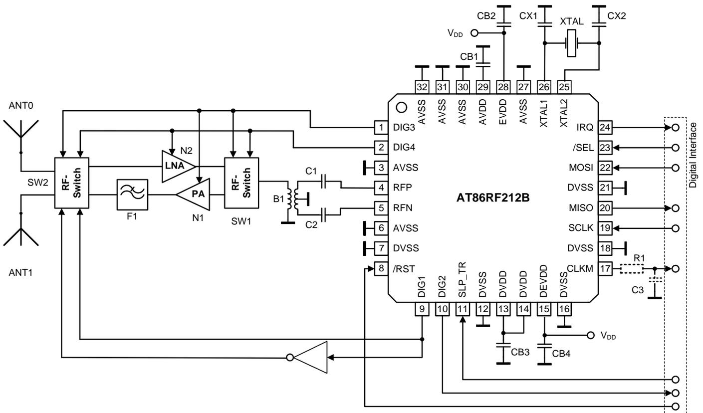
In this example, a balun (B1) transforms the differential RF signal at the Atmel AT86RF212B radio transceiver RF pins (RFP/RFN) to a single ended RF signal, similar to the Basic Application Schematic; refer to [Figure 5-1](#). The RF switches (SW1, SW2) separate between receive and transmit path in an external RF front-end. These switches are controlled by the RX/TX Indicator, represented by the differential pin pair DIG3/DIG4; refer to [Section 11.4](#).
