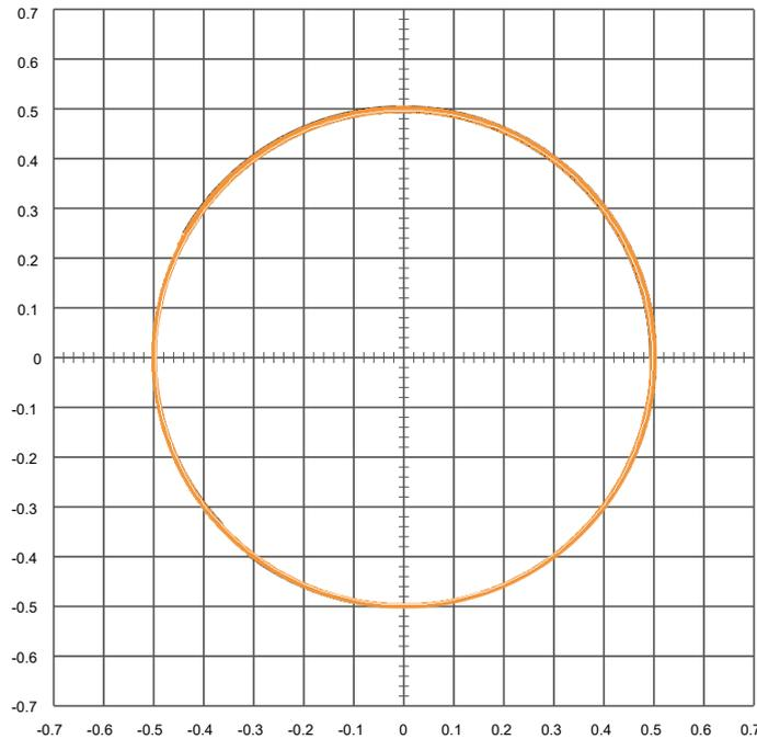
Figure 3. Lissajous curve of the measured X-Y signals
