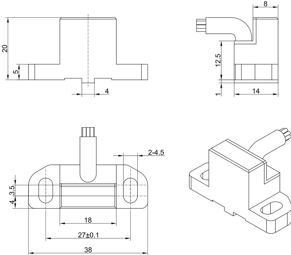
Figure 7. Outline of GE series encoder (unit: mm)
