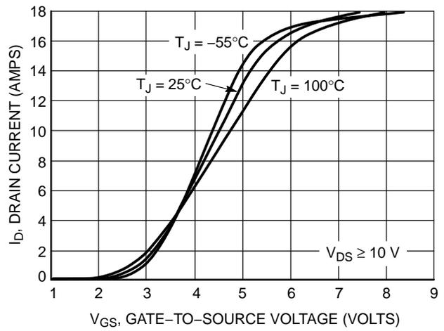
Figure 2. Transfer Characteristics
