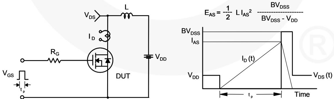
Figure 16. Unclamped Inductive Switching Test Circuit & Waveforms
