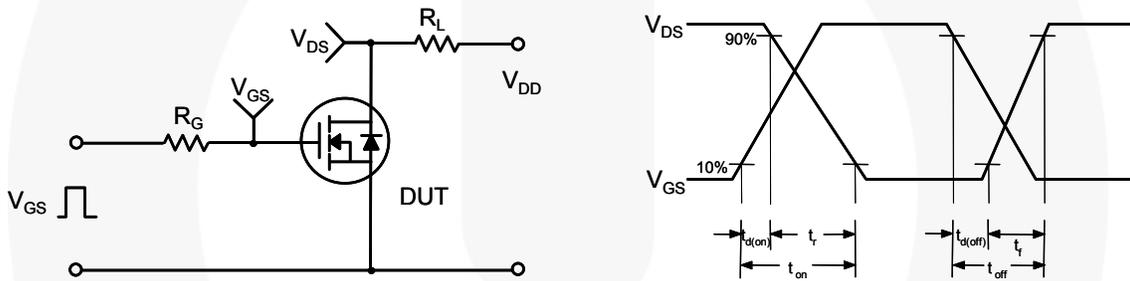
Figure 15. Resistive Switching Test Circuit & Waveforms
