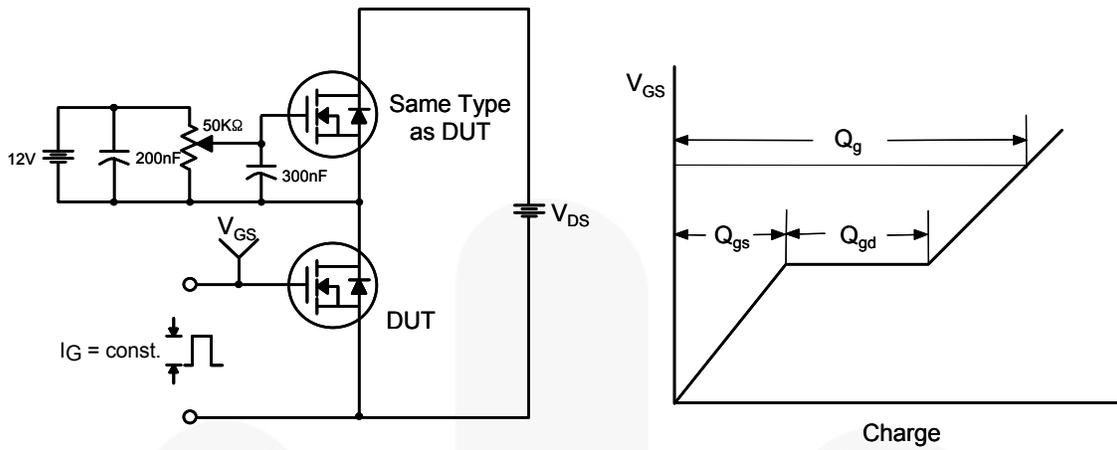
Figure 14. Gate Charge Test Circuit & Waveform
