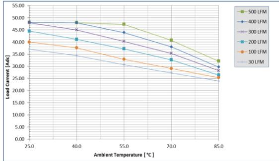
Fig. 4: Power derating vs. ambient air temperature and airflow rates for UIQ48T48050 converter w/o baseplate mounted vertically with air flowing from pin 3 to pin 1, MOSFET temperature  $\leq 125^{\circ}\text{C}$ ,  $V_{in}=24\text{V}$
