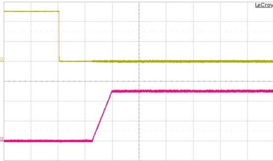
Fig. 10: Turn-on transient at full rated load current (resistive) plus 6000 $\mu$ F at  $V_{in}$  = 48 V, triggered via ON/OFF pin. Top trace: ON/OFF signal (2V/div.). Bottom trace: output voltage (2V/div.). Time scale: 50 ms/div.
