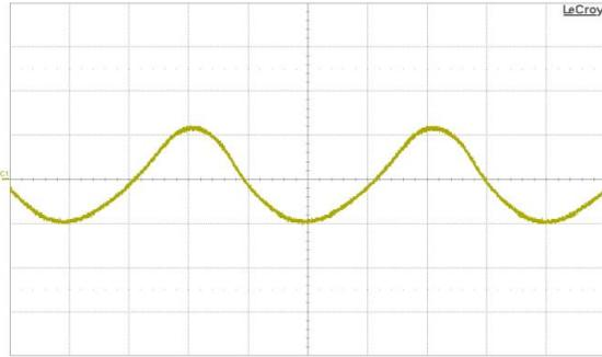
Fig. 16: Input reflected ripple current,  $i_s$  (20 mA/div.), measured through 10  $\mu$ H at the source at full rated load current and  $V_{in} = 48$  V. Refer to Fig. 14 for test setup. Time scale: 1  $\mu$ s/div.
