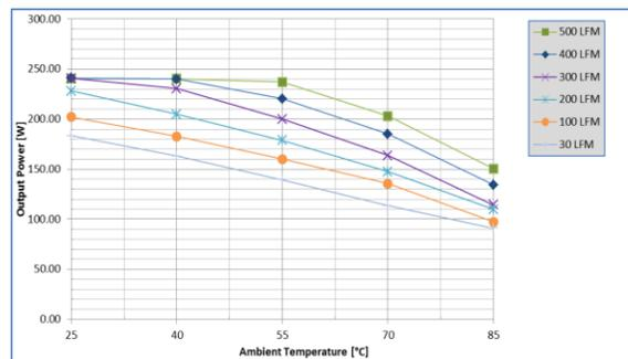
Fig. 3: Available load current vs. ambient air temperature and airflow rates for UIQ48T48050 converter w/o baseplate mounted vertically with air flowing from pin 3 to pin 1, MOSFET temperature  $\leq 125^{\circ}\text{C}$ ,  $V_{in}=24\text{V}$
