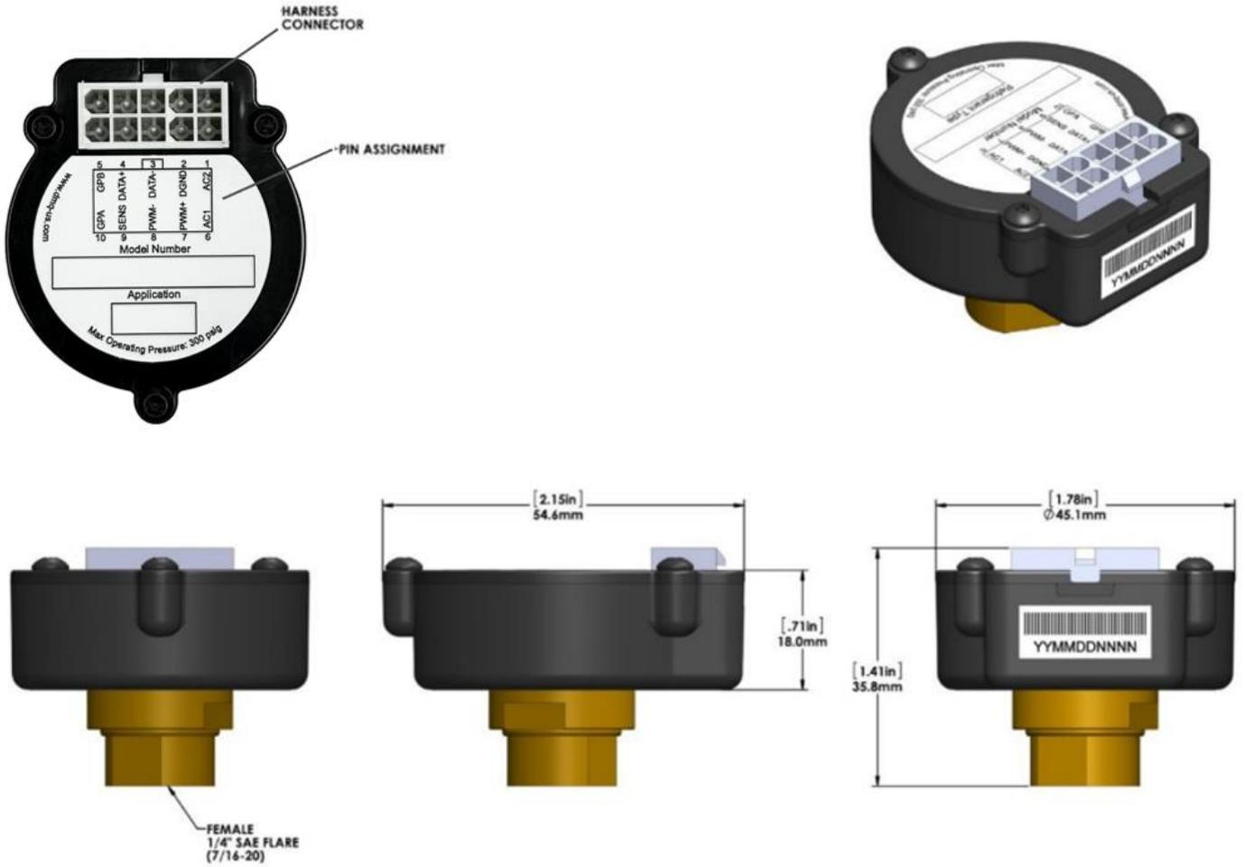
Figure 3: DPTS Physical dimensions and Product markings
