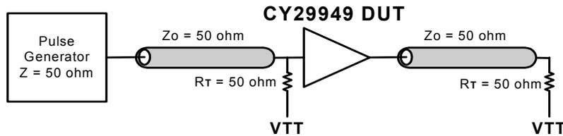
Figure 3. PECL\_CLK CY29949 Test Reference for  $V_{CC} = 3.3V$  and  $V_{CC} = 2.5V$
